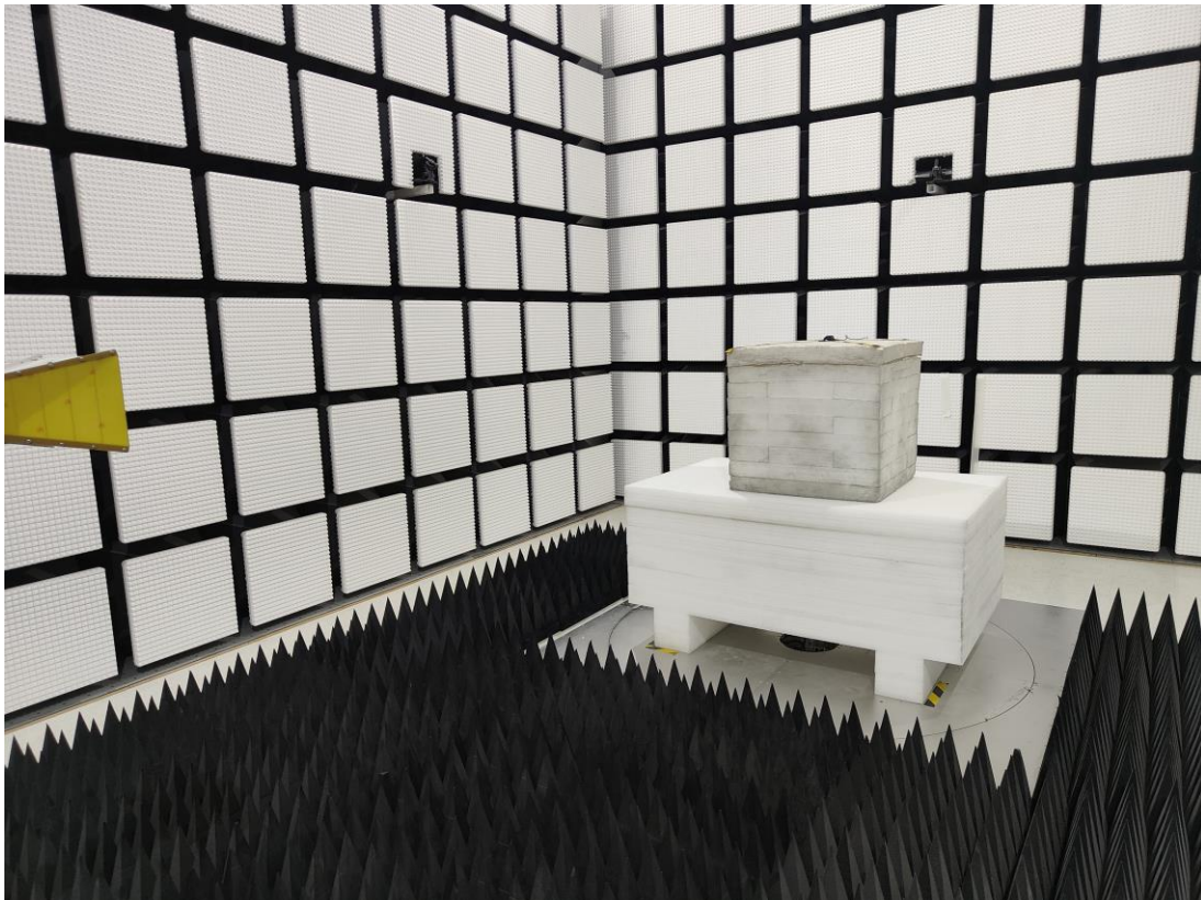
Radiated Emission Above 1GHz View
