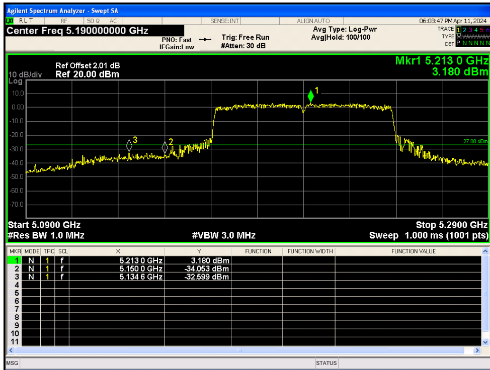
Band Edge NVNT n20 5180MHz Low Ant1
