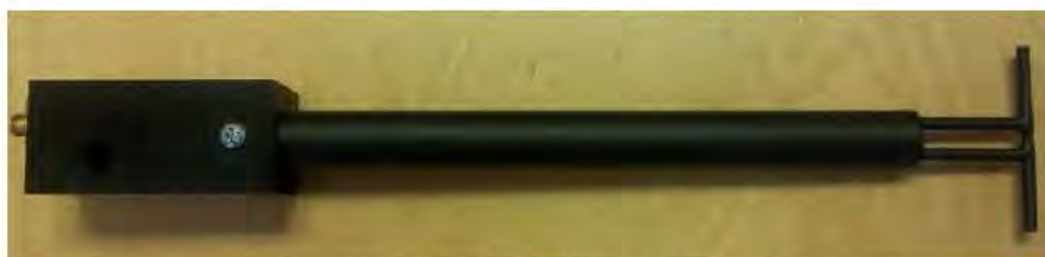
Figure 1 – MVG COMOSAR Validation Dipole
