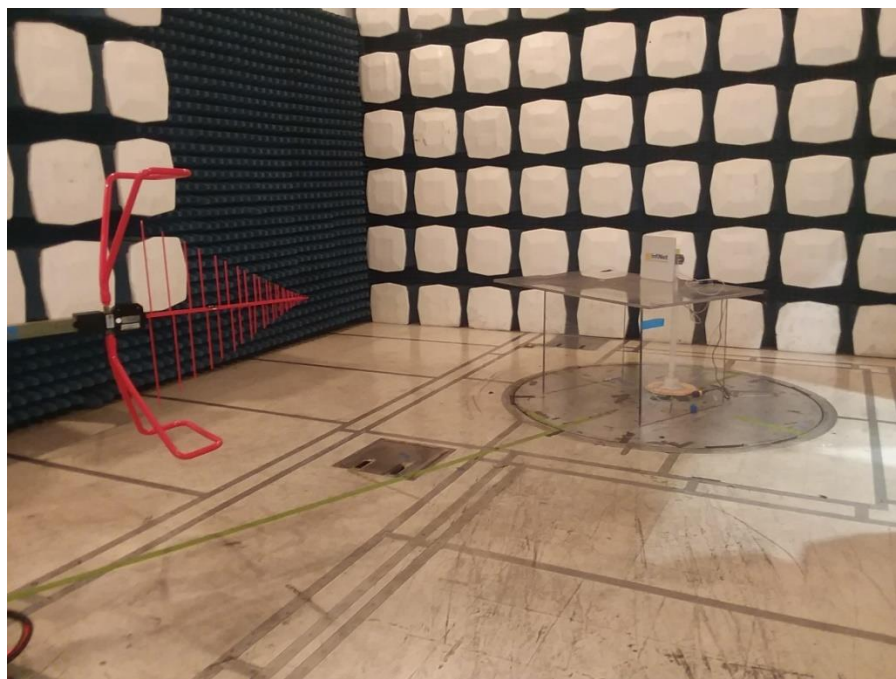
Photograph 2. Radiated Emissions Setup between 30MHz - 1GHz
