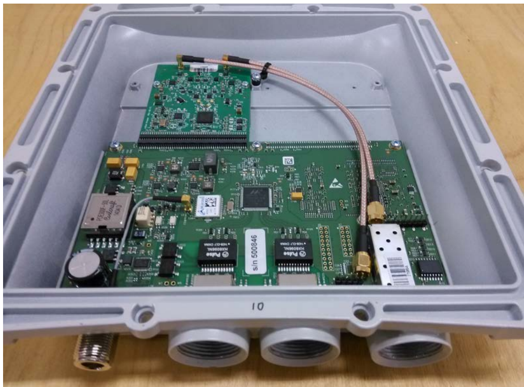
Photograph 3. The InfliLINK XG Xm/5X.500.2x500.2x23 unit (FCC ID: X8Q-XM5X), the assembled device (the antenna is not connected)
