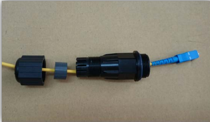
Figure 11 - SFP Connection Step 1
