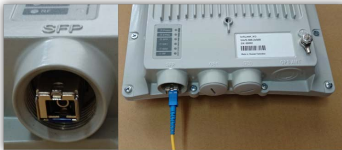
Figure 12 - SFP Connection Step 2
