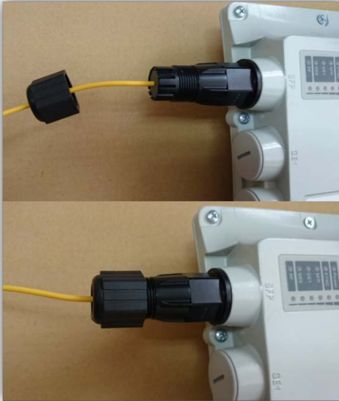
Figure 13 - SFP Connection Step 3
