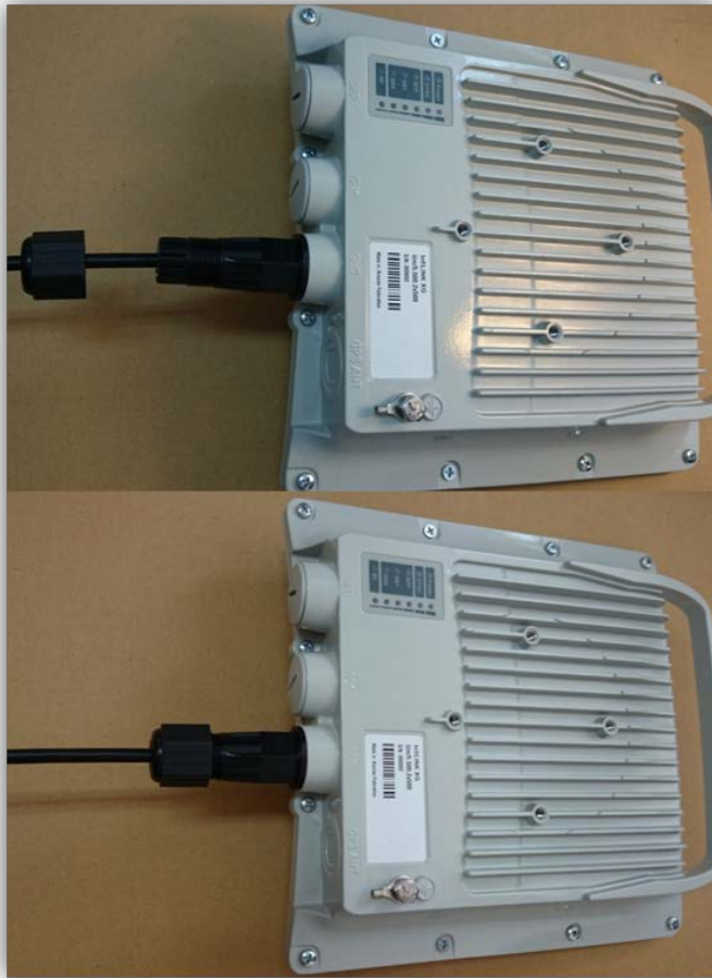
Figure 9 - RJ-45 Connection Step 2
