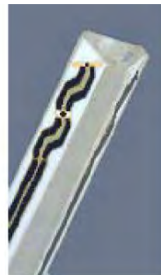
Figure 2.3 Probe Thick-Film Technique
