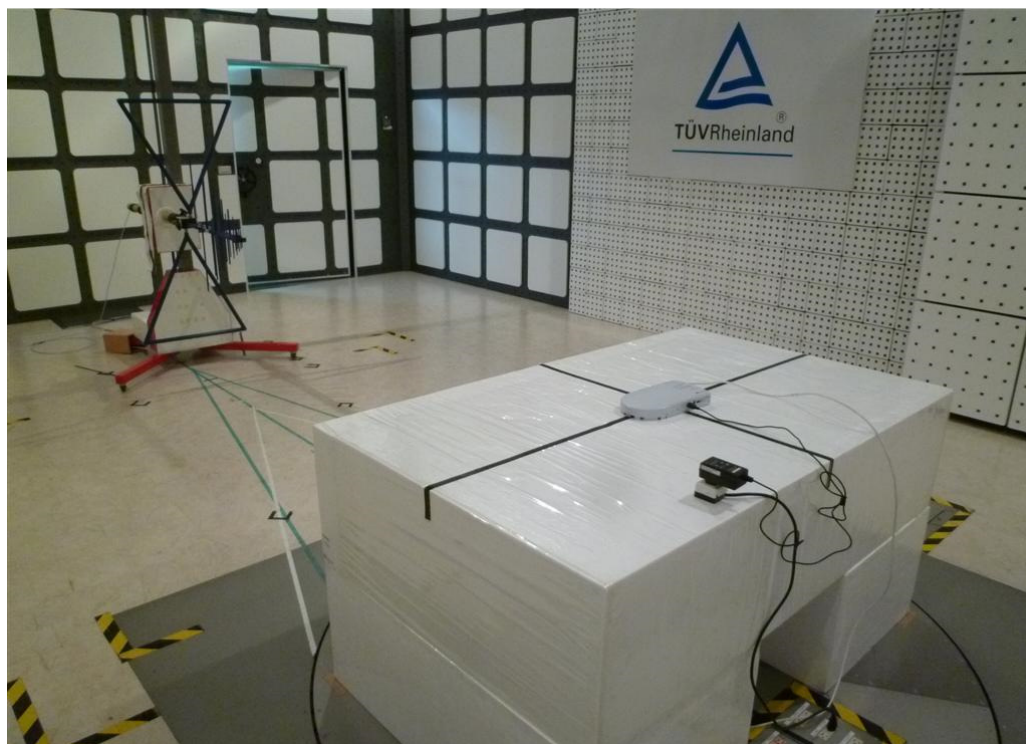
Photograph 2: Set-up for Spurious Emissions (Back View 1)
