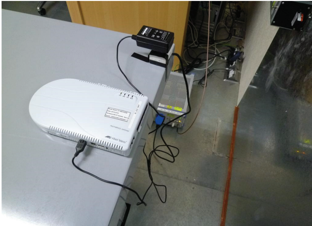
Photograph 5: Set-up for for Mains Conducted testing Back
