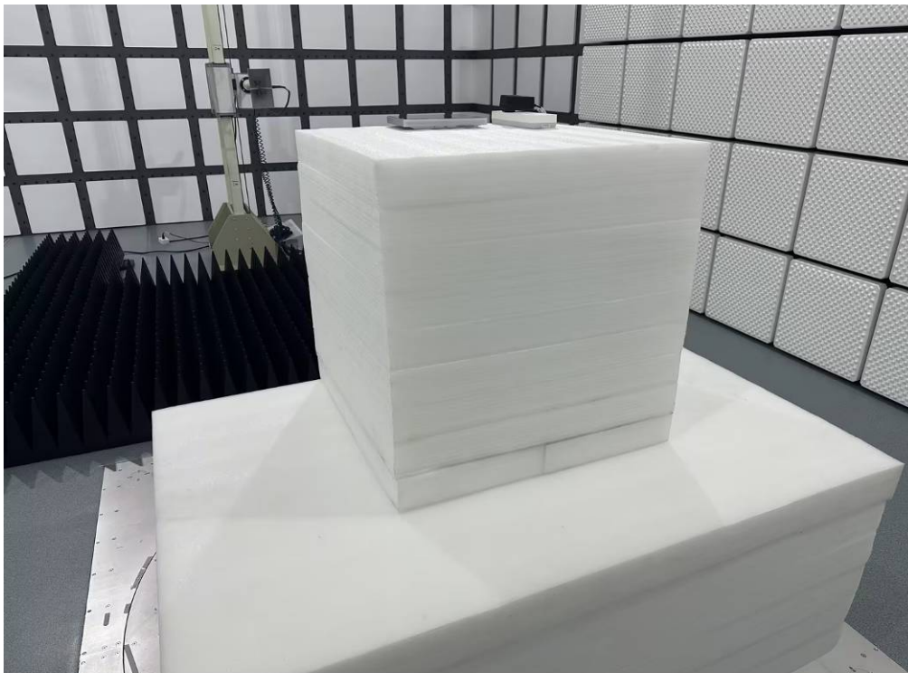
Photo of Radiated Emission Measurement (Above 1G)
