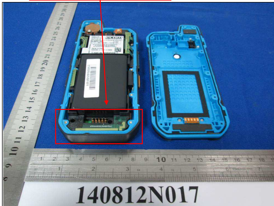
WWAN Main TX/RX Antenna
