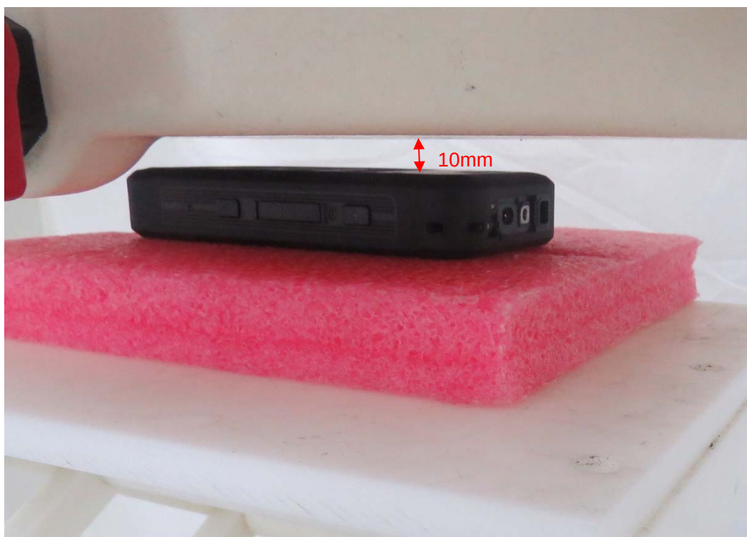
Picture 10: Back Side, the distance from handset to the bottom of the Phantom is 10mm
