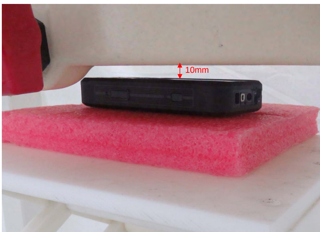
Picture 11: Front Side, the distance from handset to the bottom of the Phantom is 10mm
