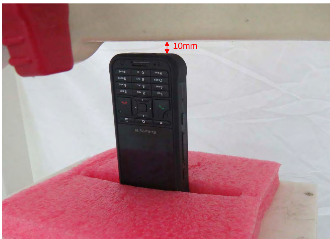
Picture 15: Bottom Side, the distance from handset to the bottom of the Phantom is 10mm
