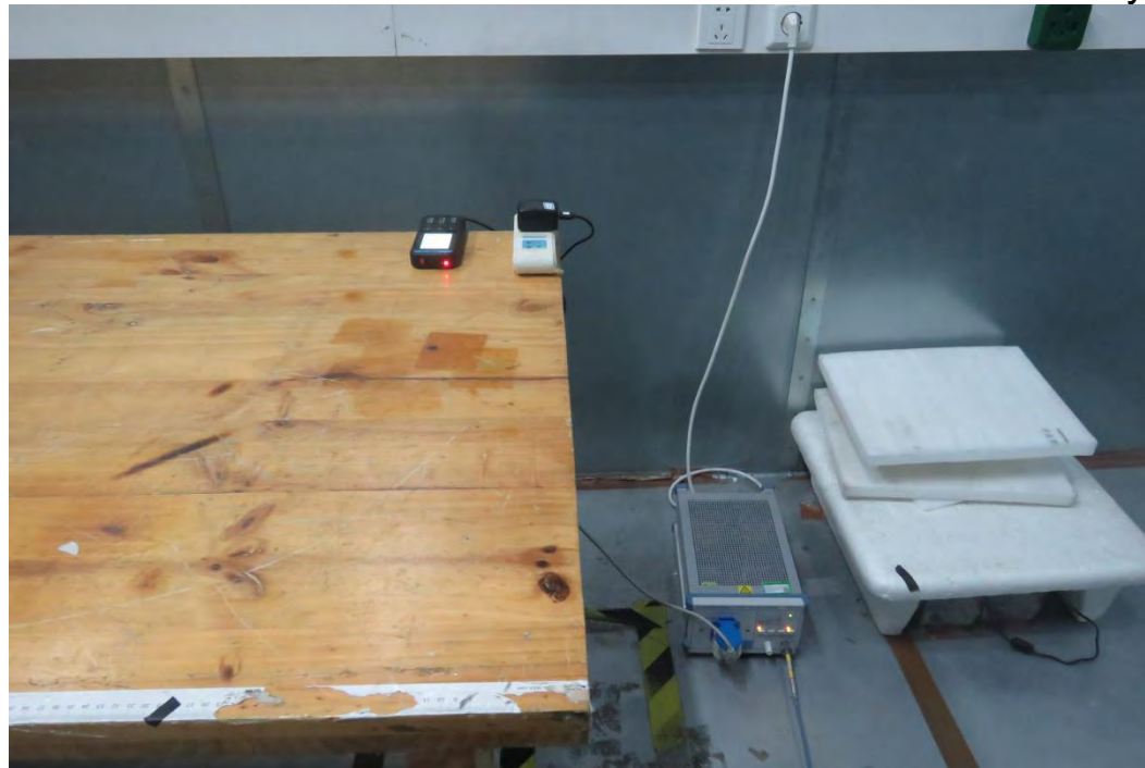
Picture 3 Conducted Emission Test Setup
