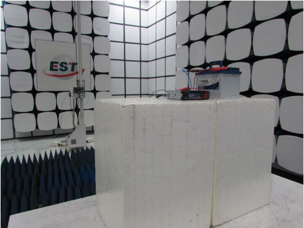
Radiated Test (Above 1GHz)
