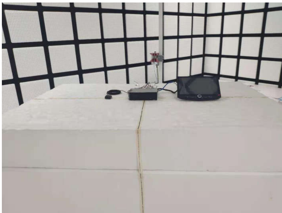
Radiated spurious emission Test Setup-3(Above 1GHz)
