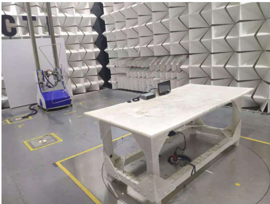
Radiated spurious emission Test Setup-2(Below 1GHz)
