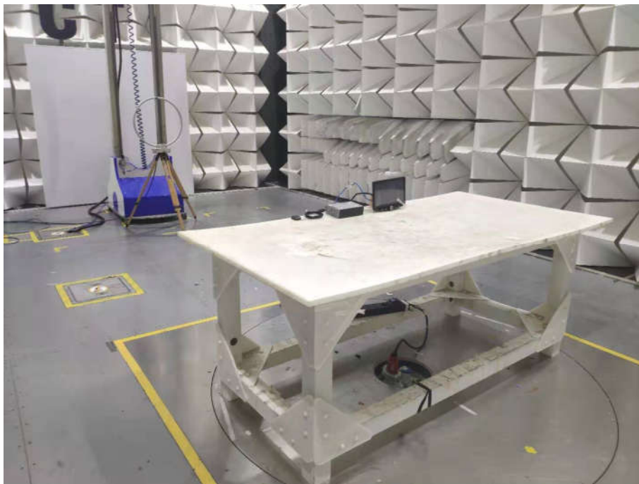
Radiated spurious emission Test Setup-1(30MHz-1GHz)
