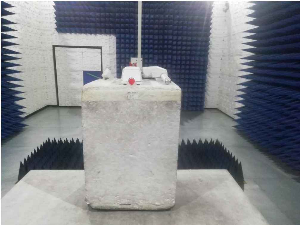
RADIATED EMISSION TEST SETUP ABOVE 1GHZ
