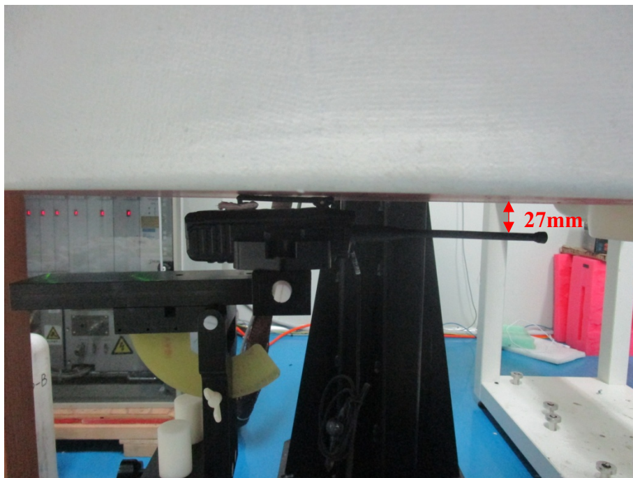
Body Worn Back Setup Photo (0mm)
