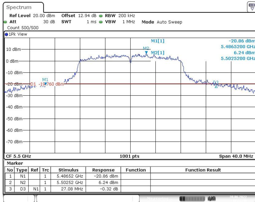
Fig. 7 Occupied 26dB Bandwidth (802.11a, 5500MHz)
