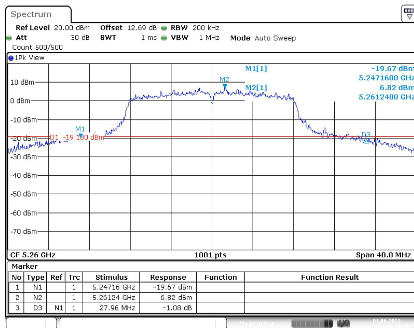
Fig. 4 Occupied 26dB Bandwidth (802.11a, 5260MHz)
