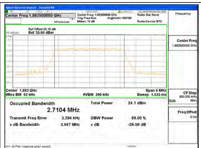
B25 / 3MHz / 256QAM/ Mid CH
