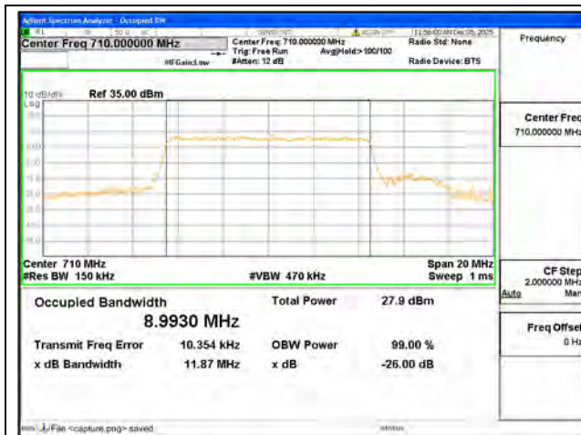
B17 / 10MHz / 64QAM/ Mid CH
