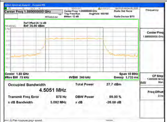
B2 / 5MHz / 16QAM/ Mid CH
