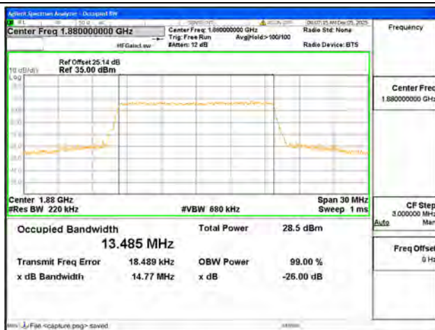
B2 / 15MHz / QPSK/ Mid CH
