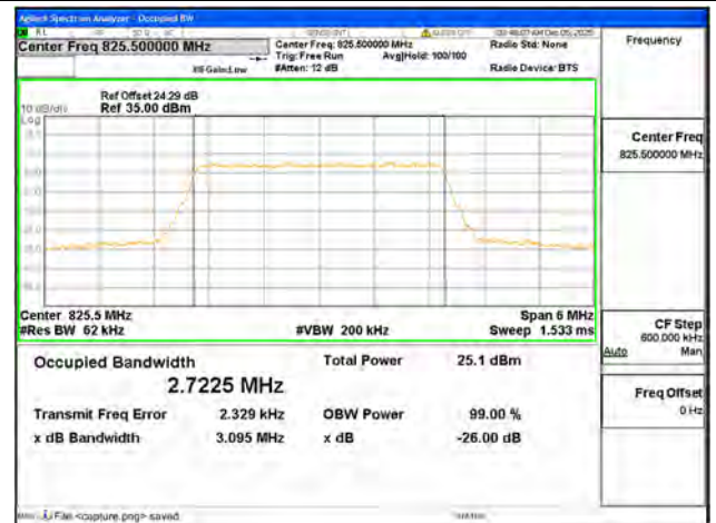
B5 / 3MHz / 256QAM/ Low CH
