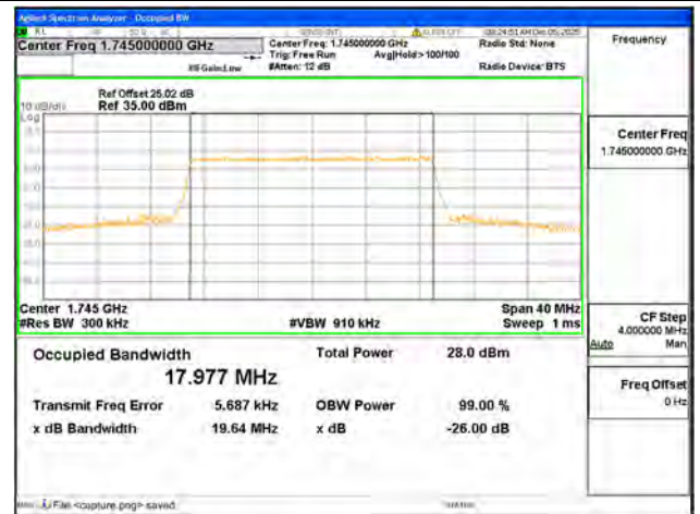
B4 / 20MHz / 16QAM/ High CH
