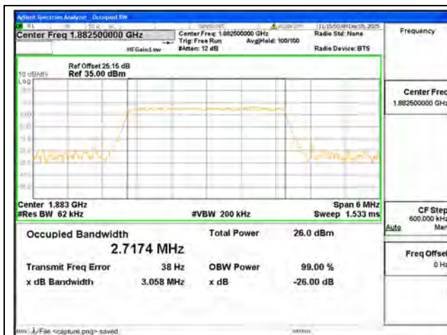
B25 / 3MHz / 64QAM/ Mid CH
