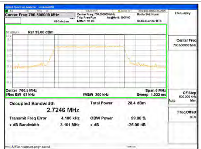
B12 / 3MHz / 16QAM/ Low CH
