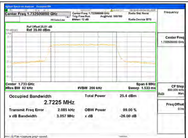
B4 / 3MHz / 256QAM/ Mid CH
