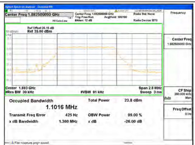
B25 / 1.4MHz / 256QAM/ Mid CH
