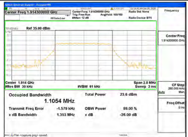
B25 / 1.4MHz / 256QAM/ High CH
