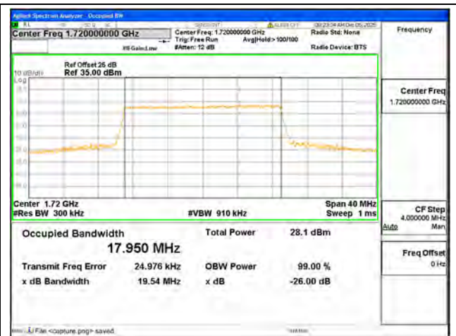
B4 / 20MHz / 16QAM/ Low CH
