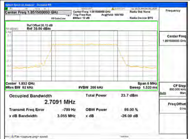
B25 / 3MHz / 256QAM/ Low CH
