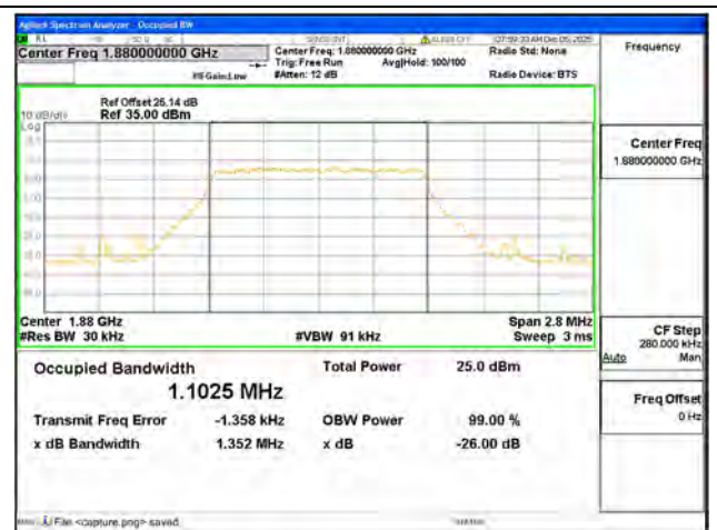
B2 / 1.4MHz / 256QAM/ Mid CH
