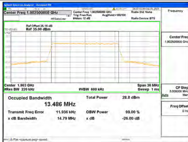
B2 / 15MHz / QPSK/ High CH
