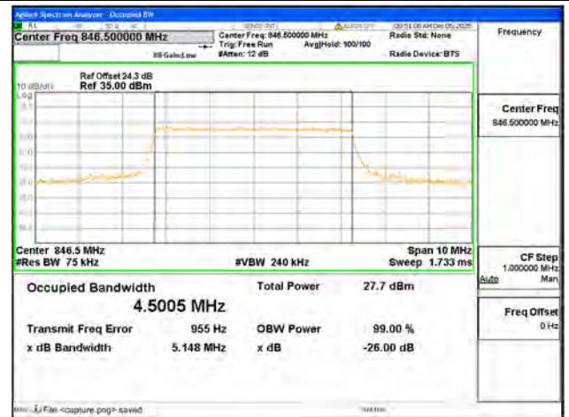
B5 / 5MHz / 16QAM/ High CH
