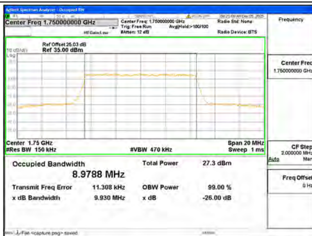
B4 / 10MHz / 64QAM/ High CH
