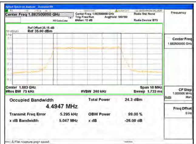
B25 / 5MHz / 256QAM/ Mid CH
