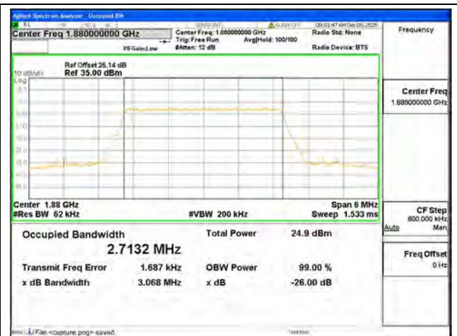
B2 / 3MHz / 256QAM/ Mid CH
