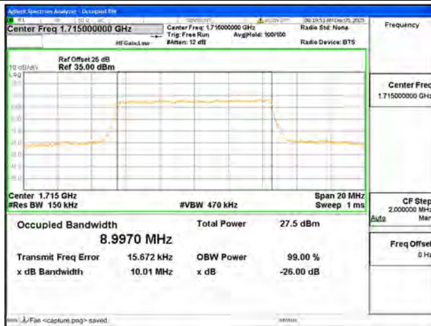
B4 / 10MHz / 64QAM/ Low CH
