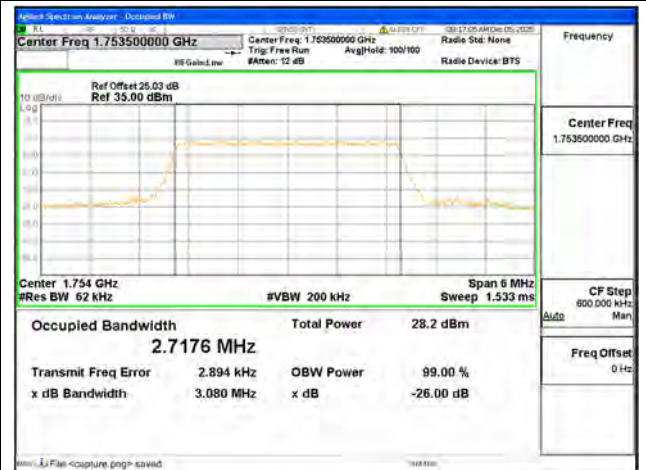
B4 / 3MHz / 16QAM/ High CH
