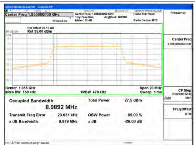
B2 / 10MHz / 16QAM/ Low CH
