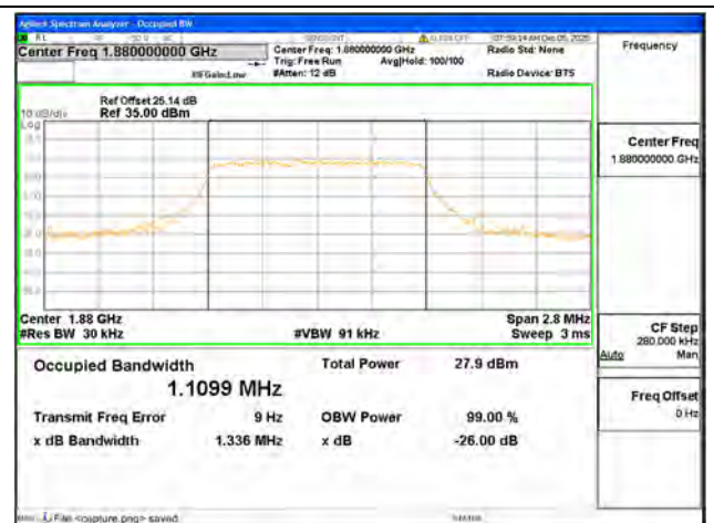
B2 / 1.4MHz / 16QAM/ Mid CH
