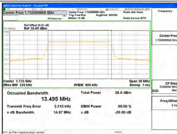
B4 / 15MHz / QPSK/ Mid CH
