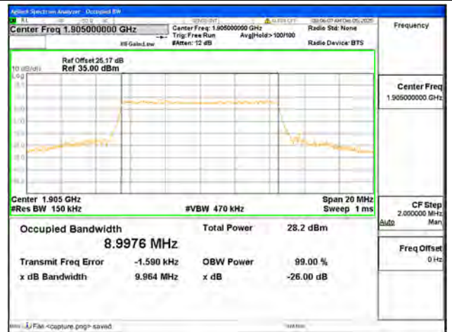
B2 / 10MHz / 16QAM/ High CH
