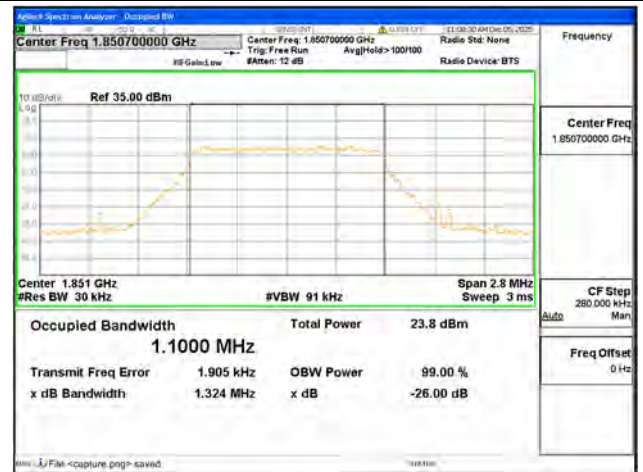
B25 / 1.4MHz / 256QAM/ Low CH
