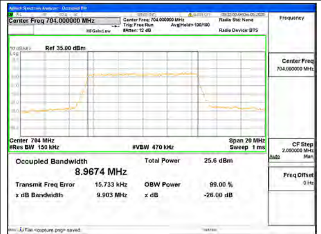
B12 / 10MHz / 256QAM/ Low CH
