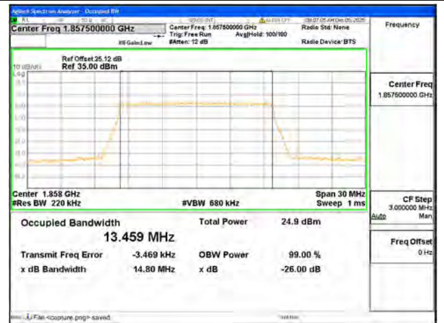
B2 / 15MHz / 256QAM/ Low CH
