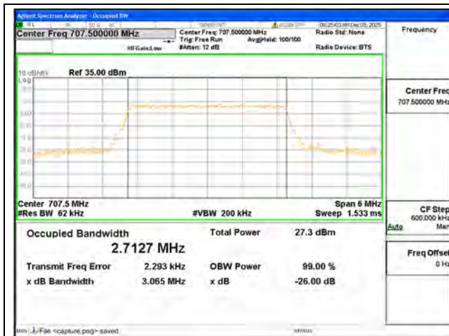
B12 / 3MHz / 64QAM/ Mid CH
