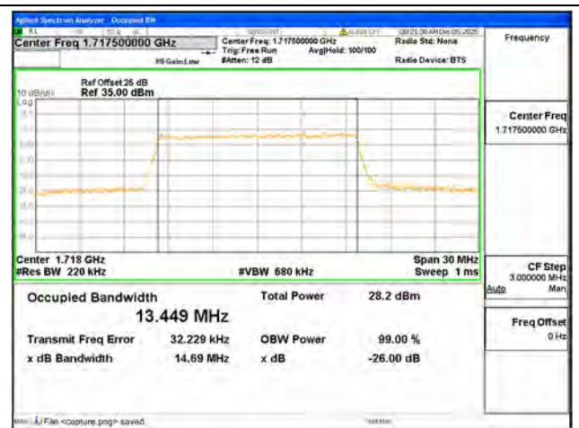
B4 / 15MHz / 16QAM/ Low CH
