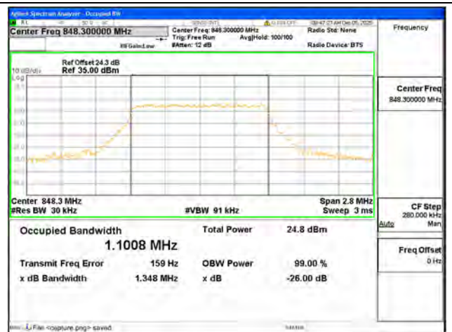
B5 / 1.4MHz / 256QAM/ High CH
