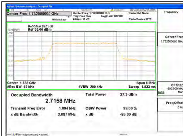
B4 / 3MHz / 64QAM/ Mid CH
