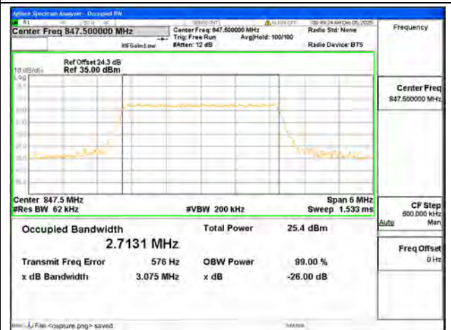
B5 / 3MHz / 256QAM/ High CH
