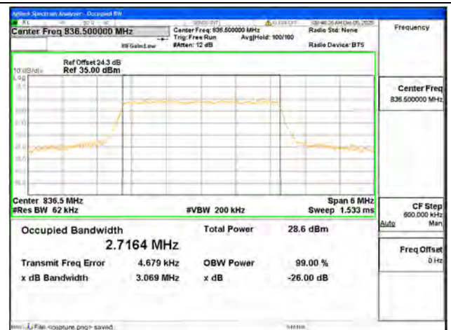
B5 / 3MHz / 16QAM/ Mid CH
