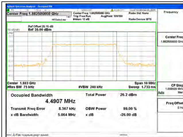
B25 / 5MHz / 64QAM/ Mid CH
