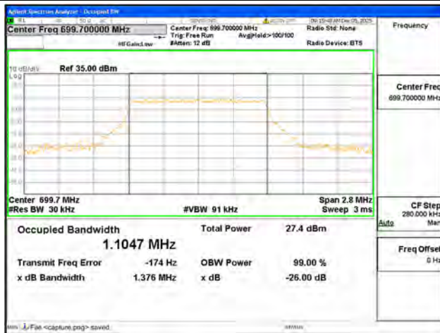
B12 / 1.4MHz / 64QAM/ Low CH
