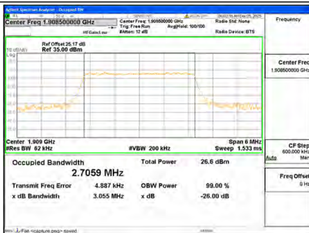
B2 / 3MHz / 64QAM/ High CH
