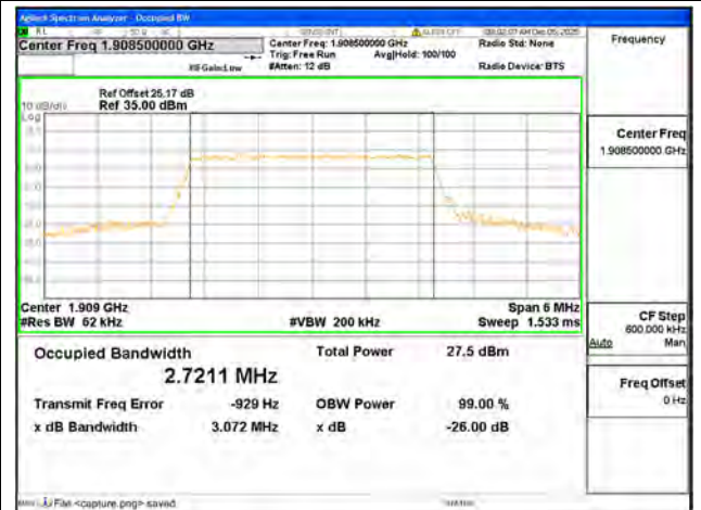
B2 / 3MHz / 16QAM/ High CH
