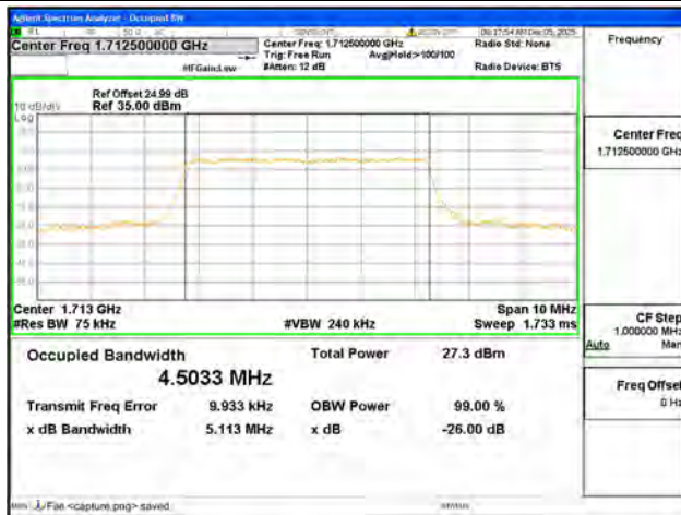
B4 / 5MHz / 64QAM/ Low CH
