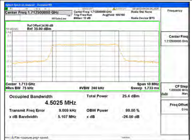
B4 / 5MHz / 256QAM/ Low CH
