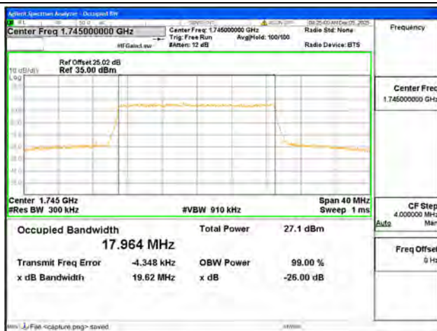
B4 / 20MHz / 64QAM/ High CH
