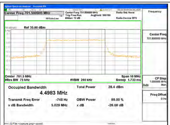
B12 / 5MHz / 16QAM/ Low CH
