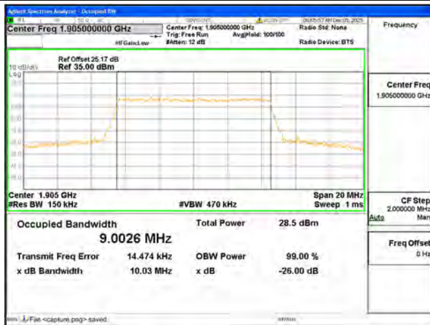
B2 / 10MHz / QPSK/ High CH
