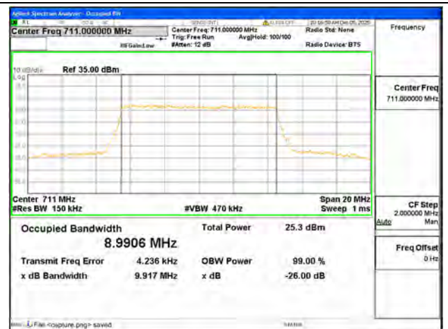
B12 / 10MHz / 256QAM/ High CH
