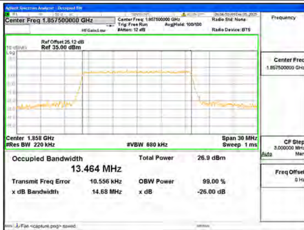
B2 / 15MHz / 64QAM/ Low CH
