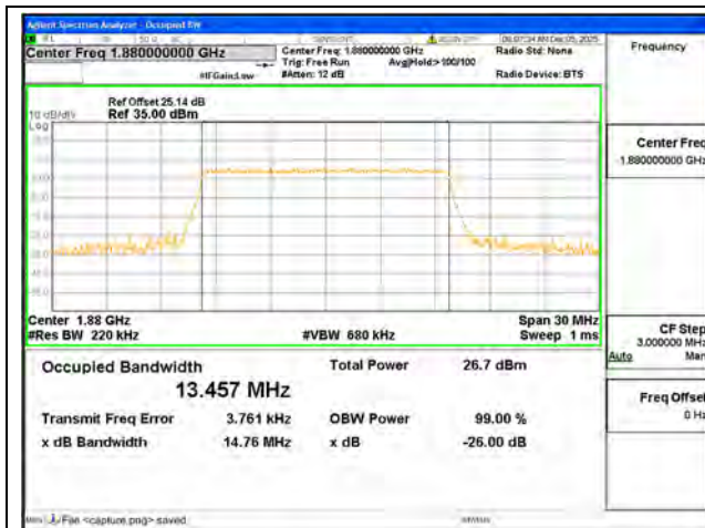
B2 / 15MHz / 64QAM/ Mid CH
