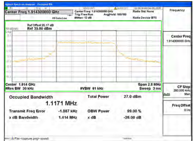
B25 / 1.4MHz / 16QAM/ High CH
