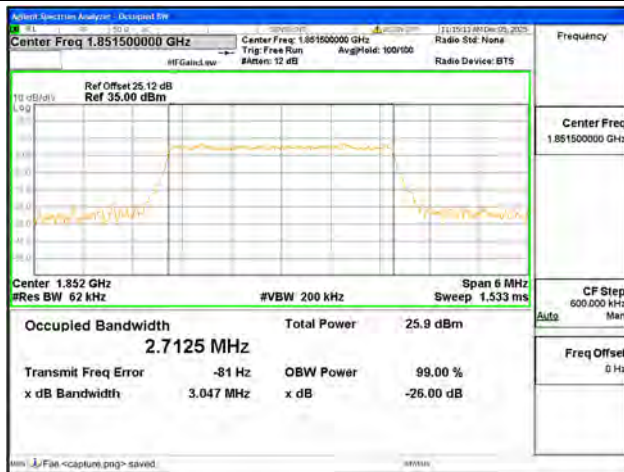
B25 / 3MHz / 64QAM/ Low CH
