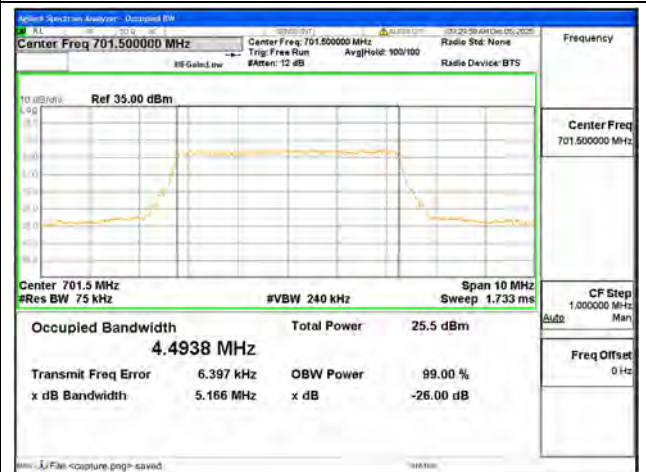
B12 / 5MHz / 256QAM/ Low CH
