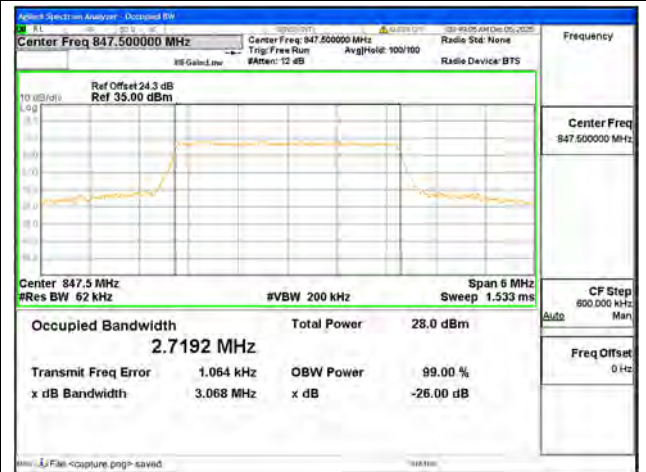
B5 / 3MHz / 16QAM/ High CH
