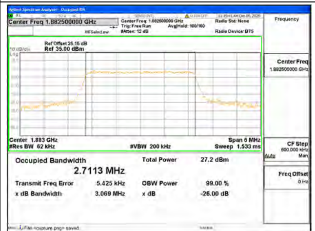
B25 / 3MHz / 16QAM/ Mid CH
