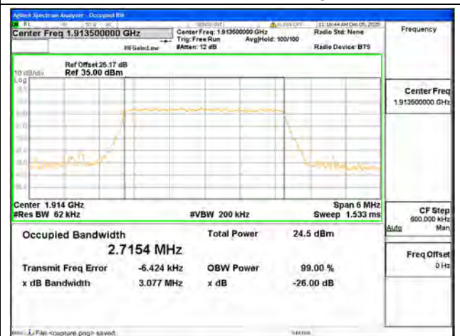
B25 / 3MHz / 256QAM/ High CH
