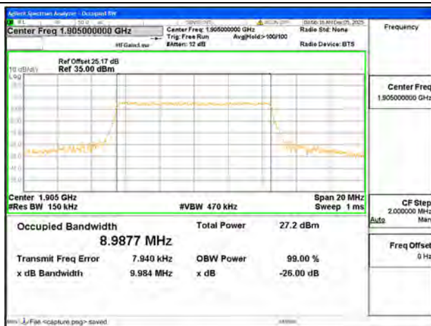
B2 / 10MHz / 64QAM/ High CH
