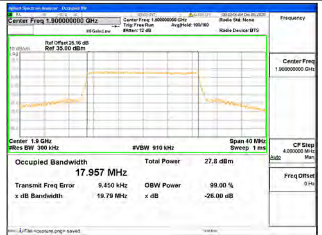
B2 / 20MHz / 16QAM/ High CH
