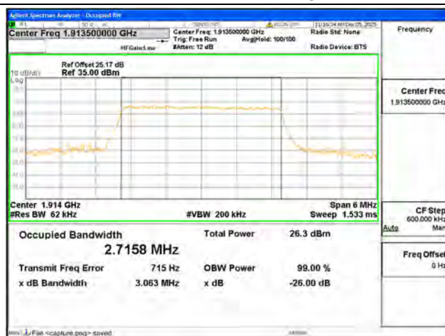
B25 / 3MHz / 64QAM/ High CH
