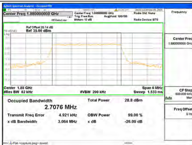
B2 / 3MHz / QPSK/ Mid CH
