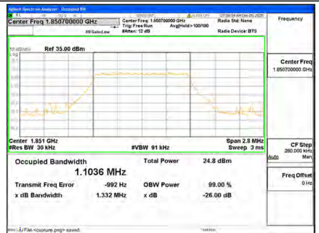
B2 / 1.4MHz / 256QAM/ Low CH
