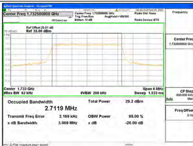
B4 / 3MHz / QPSK/ Mid CH
