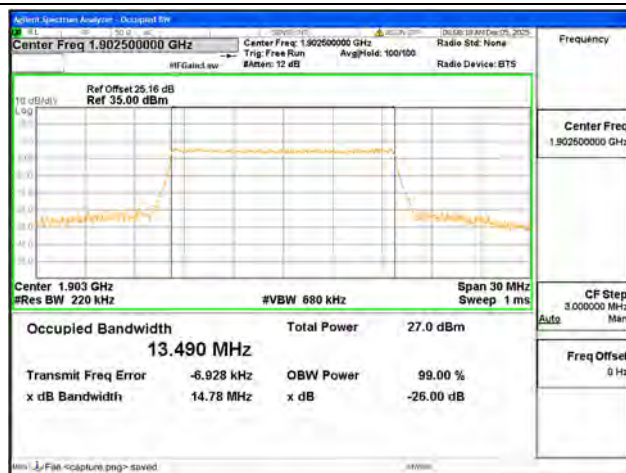
B2 / 15MHz / 64QAM/ High CH
