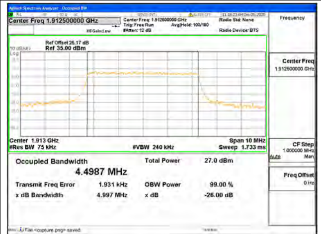
B25 / 5MHz / 16QAM/ High CH
