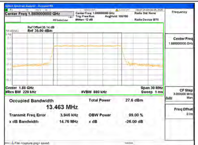
B2 / 15MHz / 16QAM/ Mid CH
