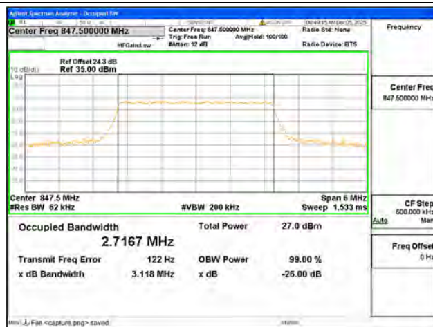
B5 / 3MHz / 64QAM/ High CH
