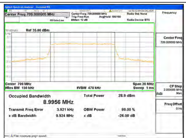
B17 / 10MHz / 16QAM/ Low CH
