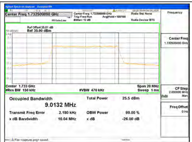
B4 / 10MHz / 256QAM/ Mid CH
