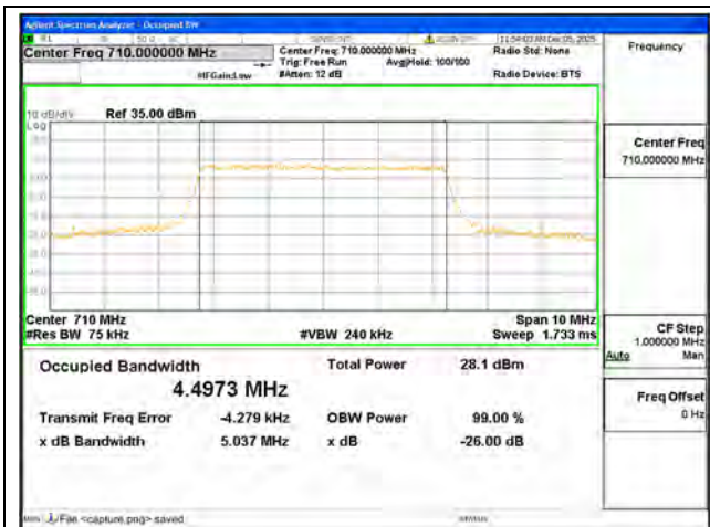
B17 / 5MHz / 64QAM/ Mid CH
