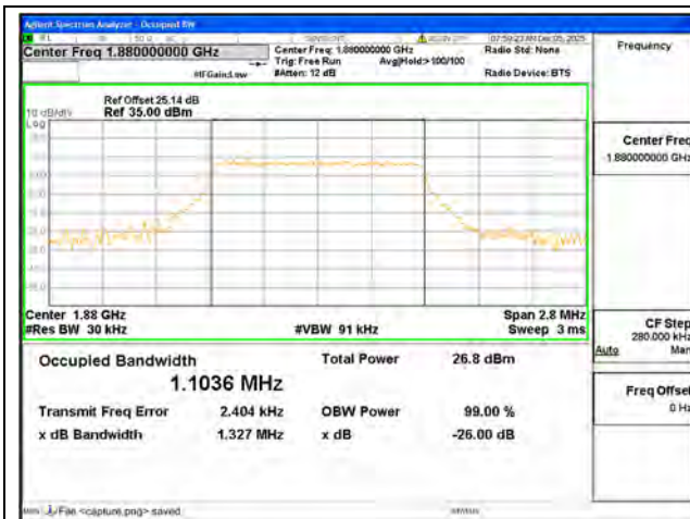
B2 / 1.4MHz / 64QAM/ Mid CH
