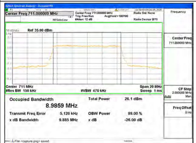
B17 / 10MHz / 256QAM/ High CH
