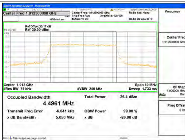
B25 / 5MHz / 64QAM/ High CH
