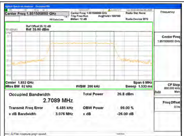
B25 / 3MHz / 16QAM/ Low CH
