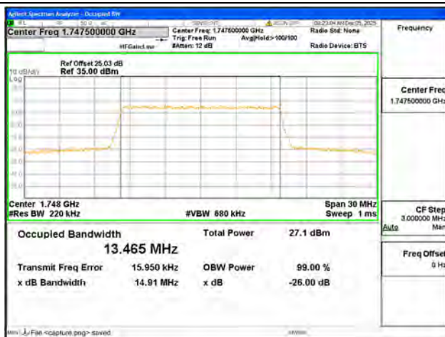
B4 / 15MHz / 64QAM/ High CH
