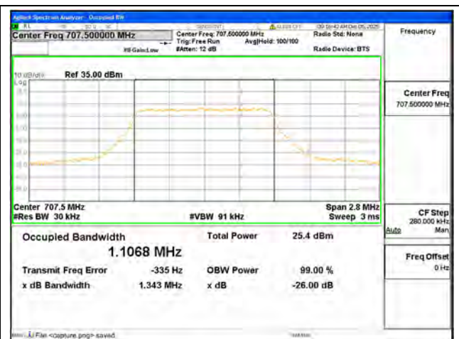
B12 / 1.4MHz / 256QAM/ Mid CH
