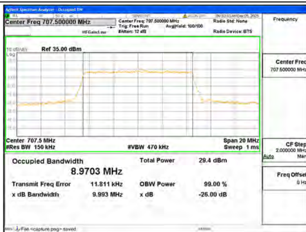
B12 / 10MHz / QPSK/ Mid CH
