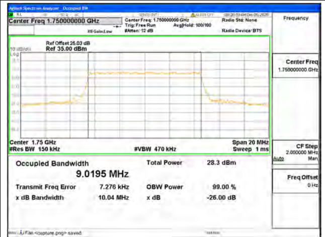
B4 / 10MHz / 16QAM/ High CH
