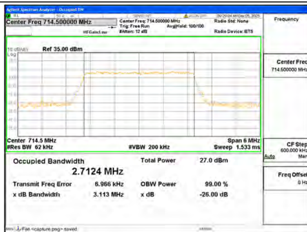
B12 / 3MHz / 64QAM/ High CH
