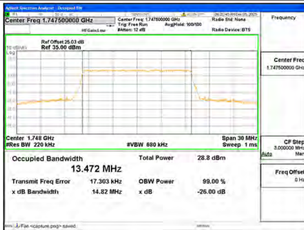
B4 / 15MHz / QPSK/ High CH
