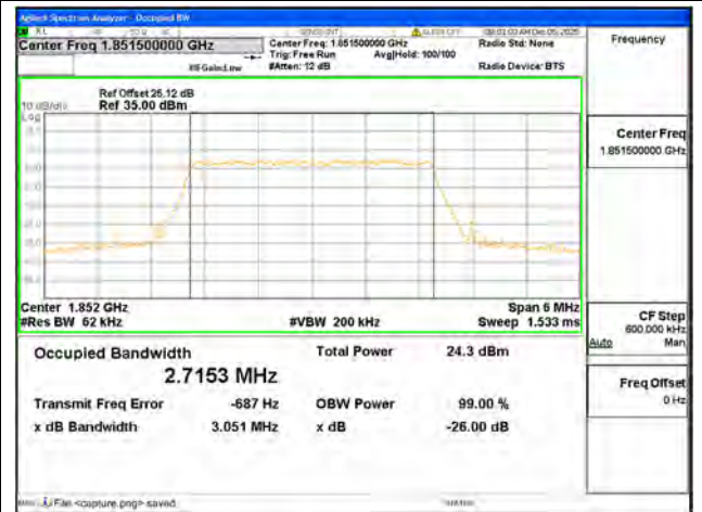
B2 / 3MHz / 256QAM/ Low CH
