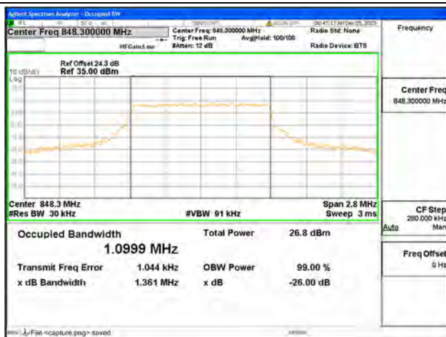
B5 / 1.4MHz / 64QAM/ High CH
