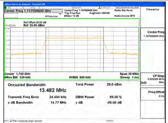
B4 / 15MHz / 16QAM/ High CH
