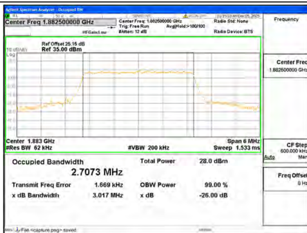
B25 / 3MHz / QPSK/ Mid CH
