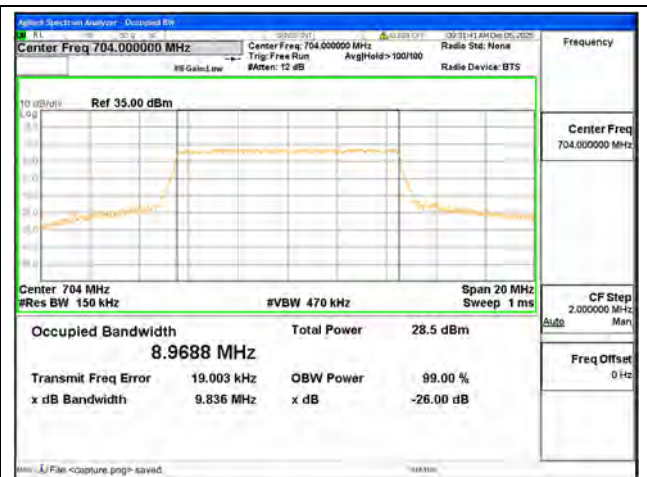
B12 / 10MHz / 16QAM/ Low CH
