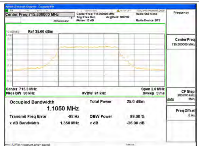
B12 / 1.4MHz / 256QAM/ High CH
