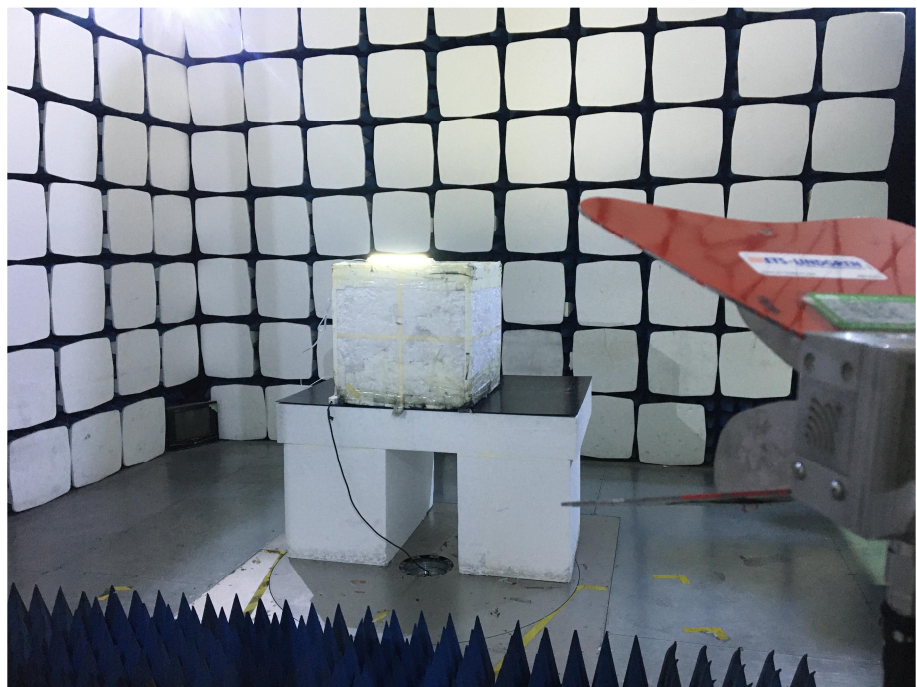
Radiation Emission Test Setup (1GHz to 18GHz)
