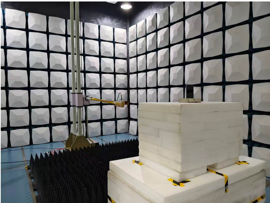
Radiated Emission 18-26.5GHz View
