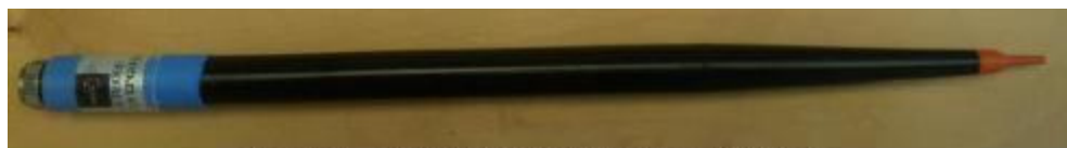
Figure 1 – MVG COMOSAR Dosimetric E-field Dipole
