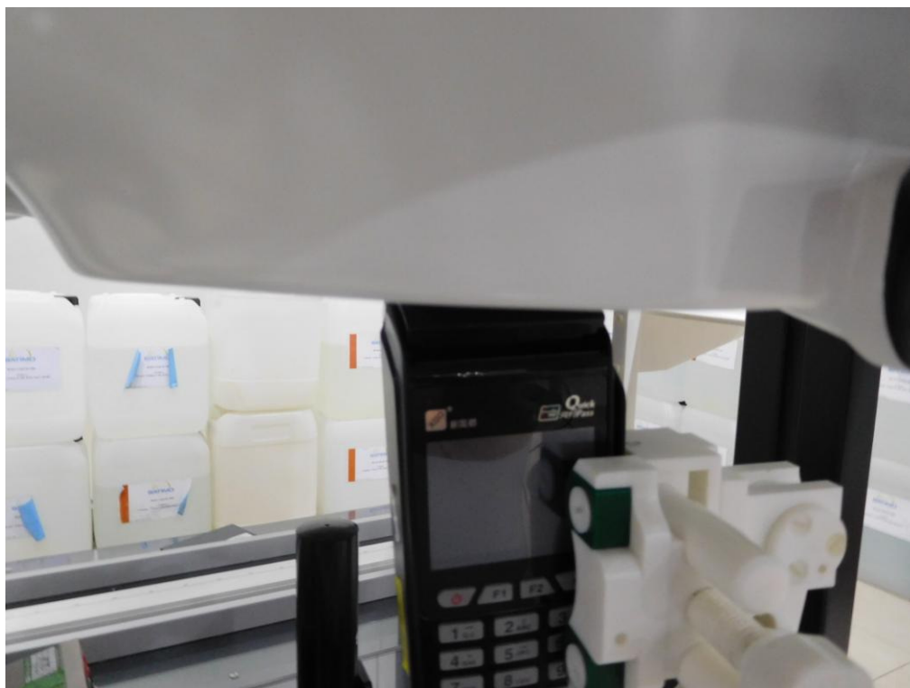
Body top side(separation distance is 0mm)
