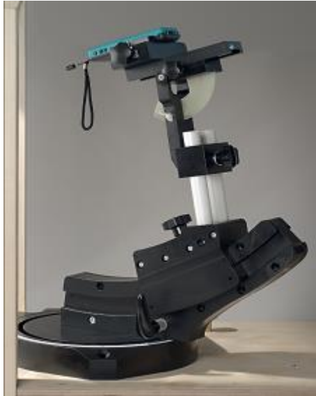
F-2. Device Holder for Transmitters
