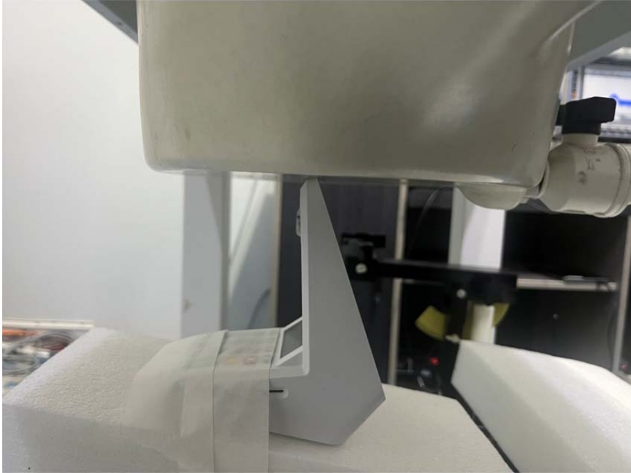
Limb Top Setup Photo(0mm)
