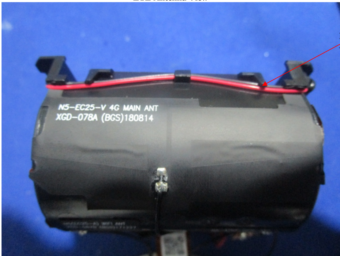
LTE Antenna View
