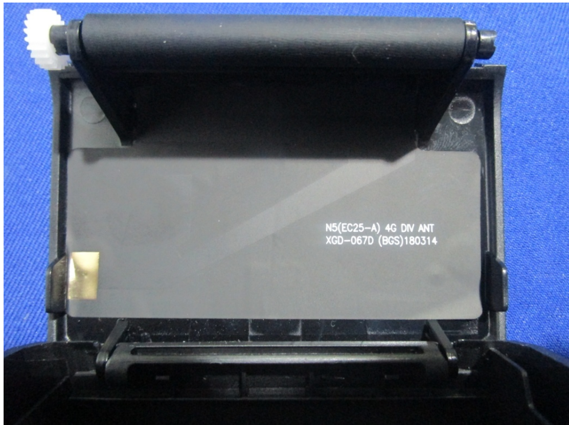
RX Antenna View
