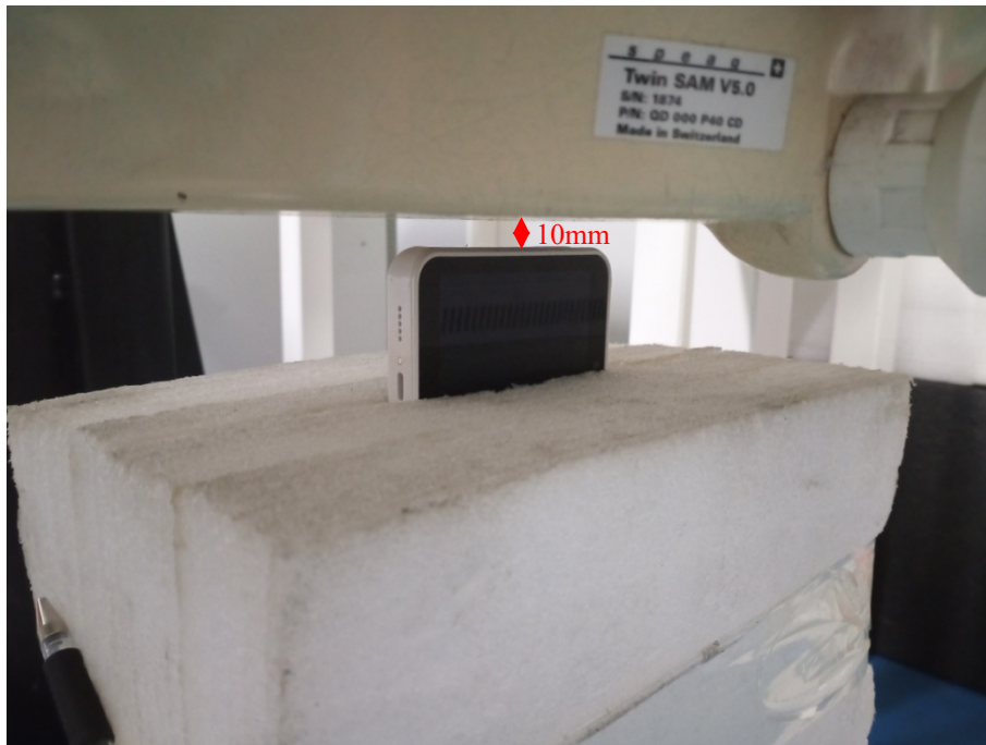
Body Left Setup Photo (10mm)
