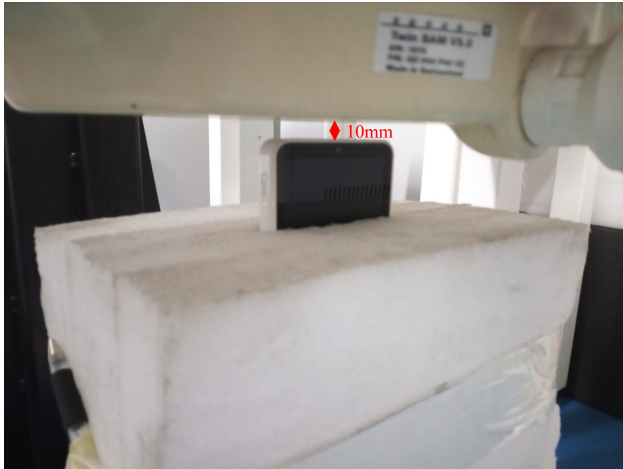
Body Top Setup Photo (10mm)
