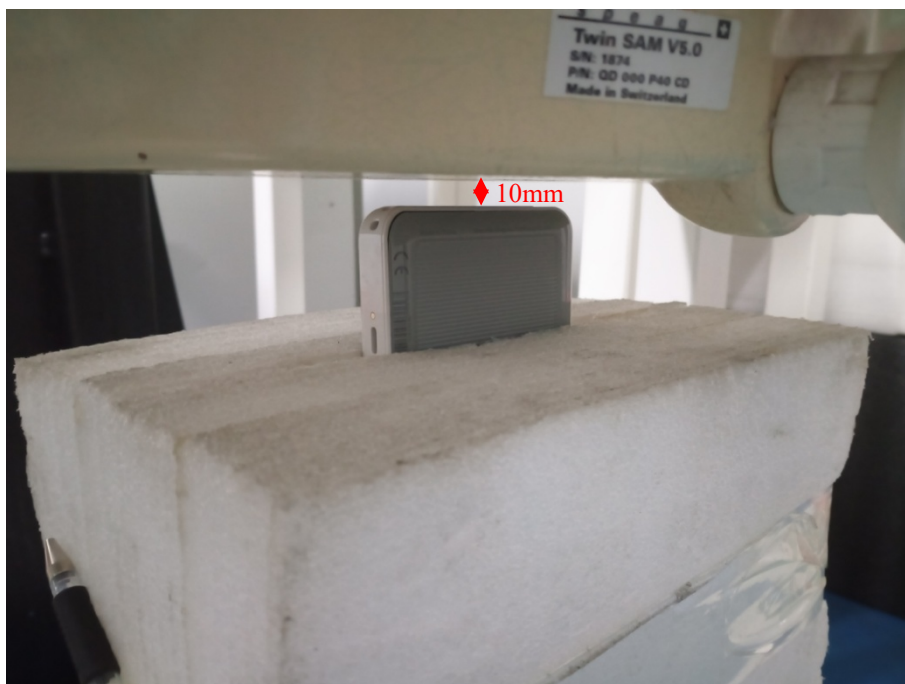
Body Right Setup Photo (10mm)
