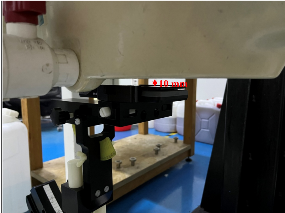
Body Back Setup Photo(10mm)
