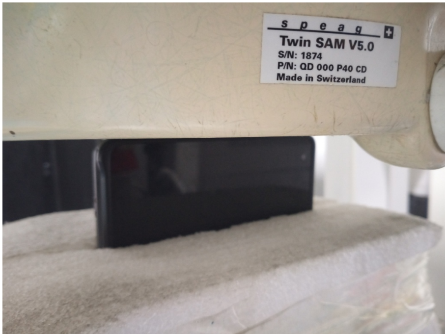
Limb Left Without Holder Setup Photo(0mm)
