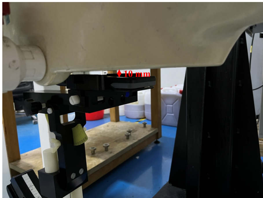
Body Front Setup Photo(10mm)
