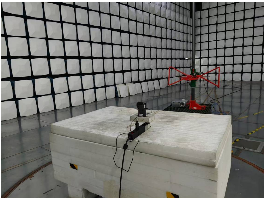
Radiated Emission 30M-1GHz View M2
