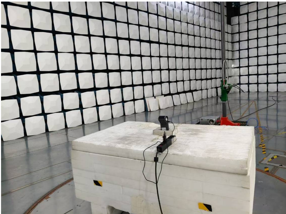
Radiated Emission 9k-30MHz Perpendicular View M2
