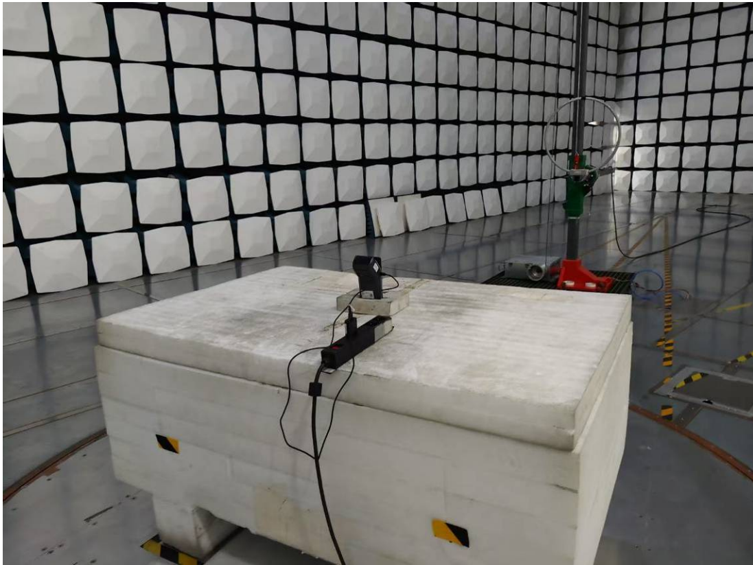
Radiated Emission 9k-30MHz Perpendicular View M2
