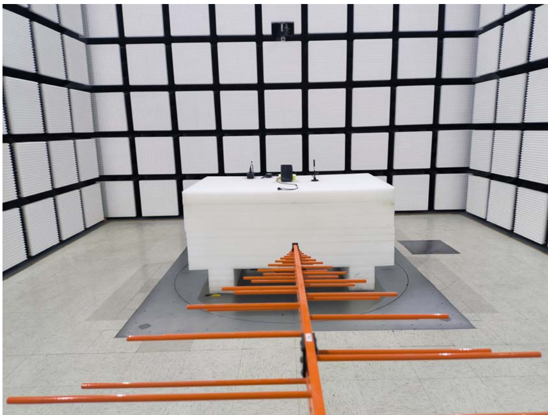
Radiated Emission 30M-1GHz View
