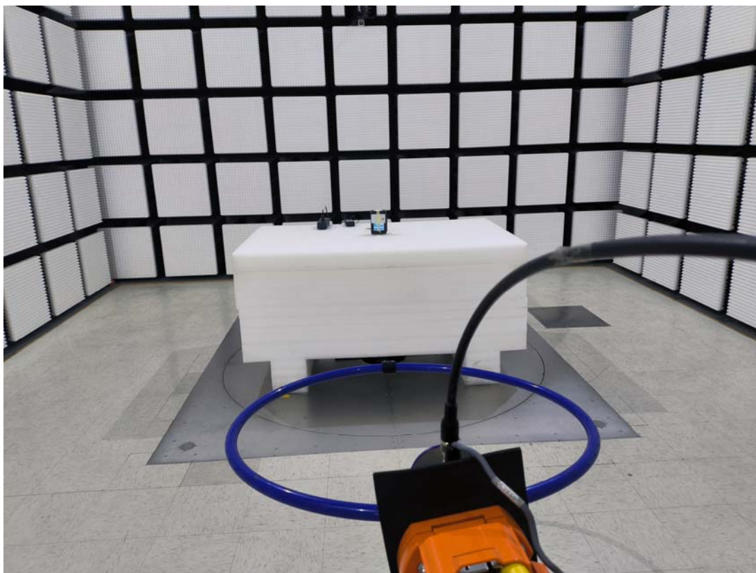
Radiated Emission 30M-1GHz View
