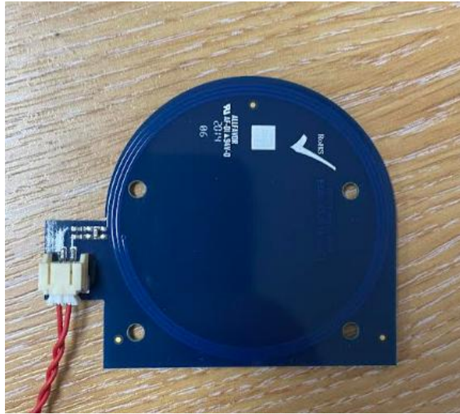
Figure 11: View of RFID Antenna removed from the product
