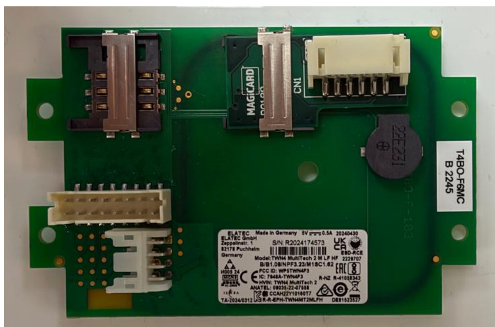
Figure 8: Top side of Elatec Smart Code Encoder PCB (PCB removed from product)
