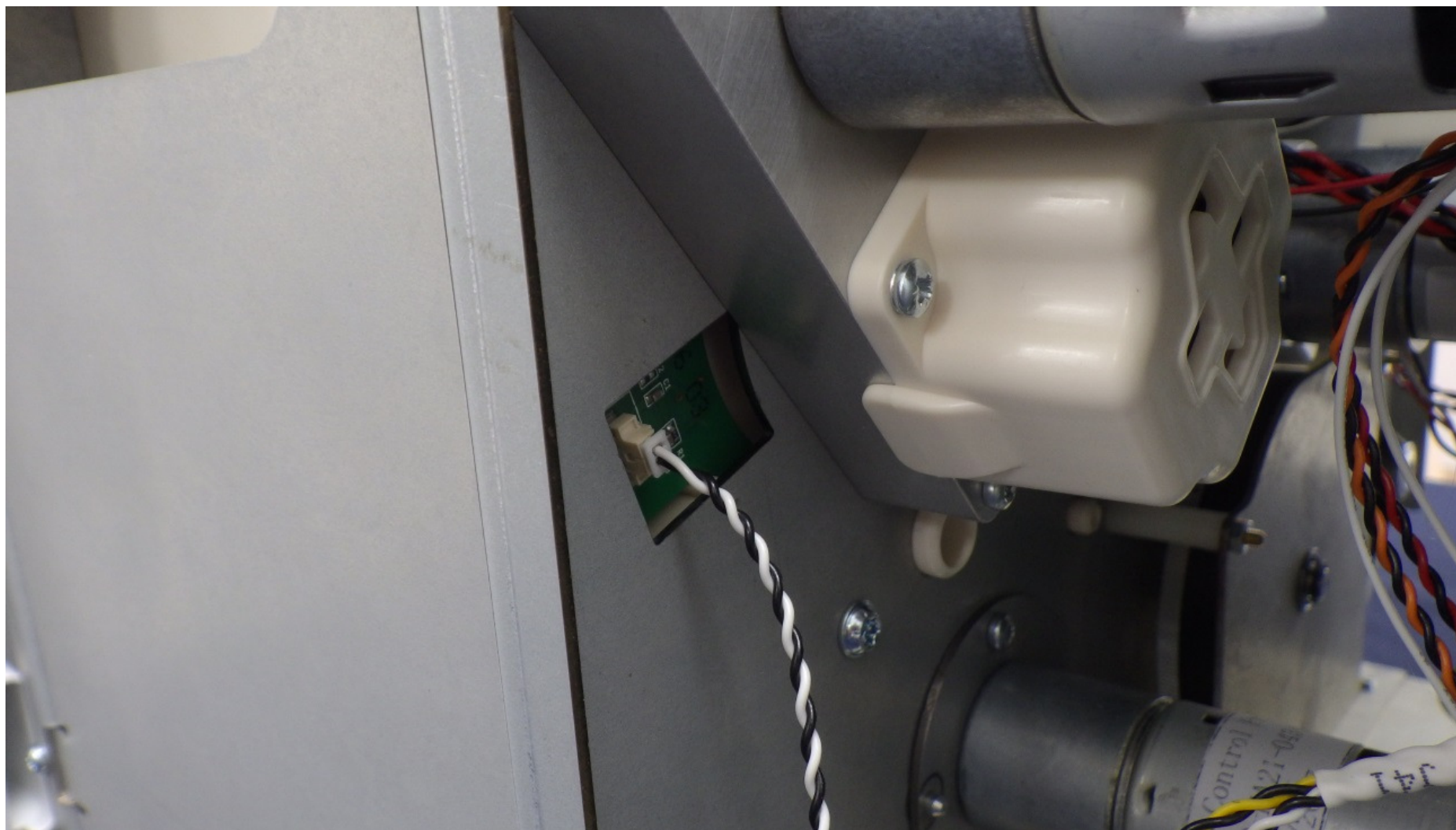
Right side view (front of product is on the left): Dye-film RFID antenna PCB connection detail (White & Black twisted pair)
