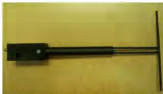
Figure 1 – MVG COMOSAR Validation Dipole
