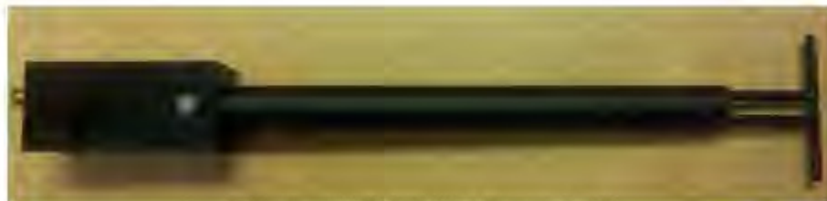
Figure 1 – MVG COMOSAR Validation Dipole
