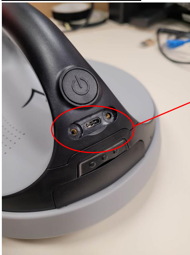
(1) Battery charging port
