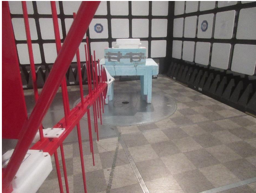
Photo 3: – Test Setup – 30MHz to 1GHz – Vertical Polarization(2.4GHz/915MHz)
