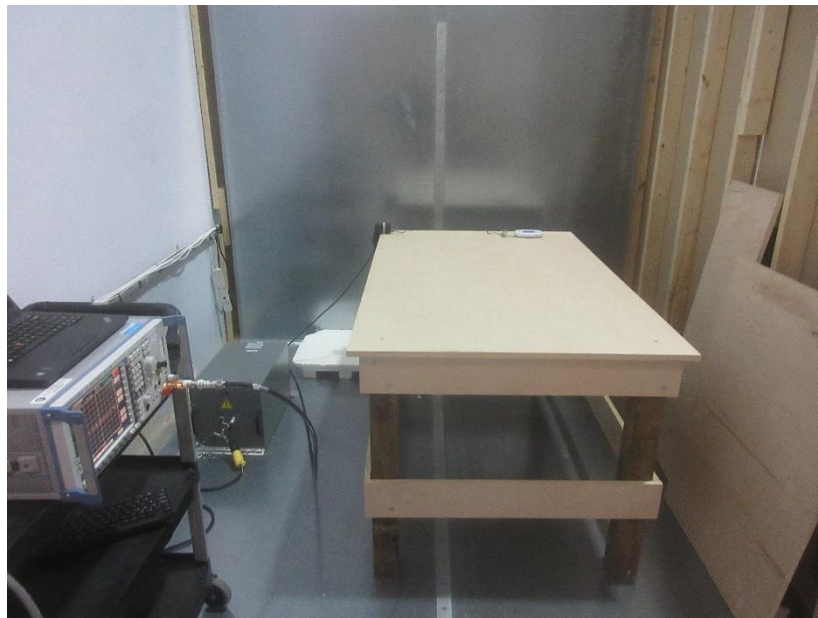
Photo 5: – Test Setup – Conducted Emission WX DB (2.4GHz/915MHz)
