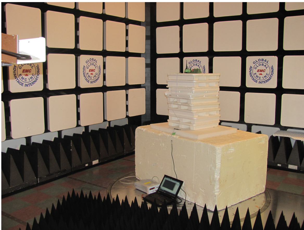
Illustration 3: Radiated setup - photo 3
