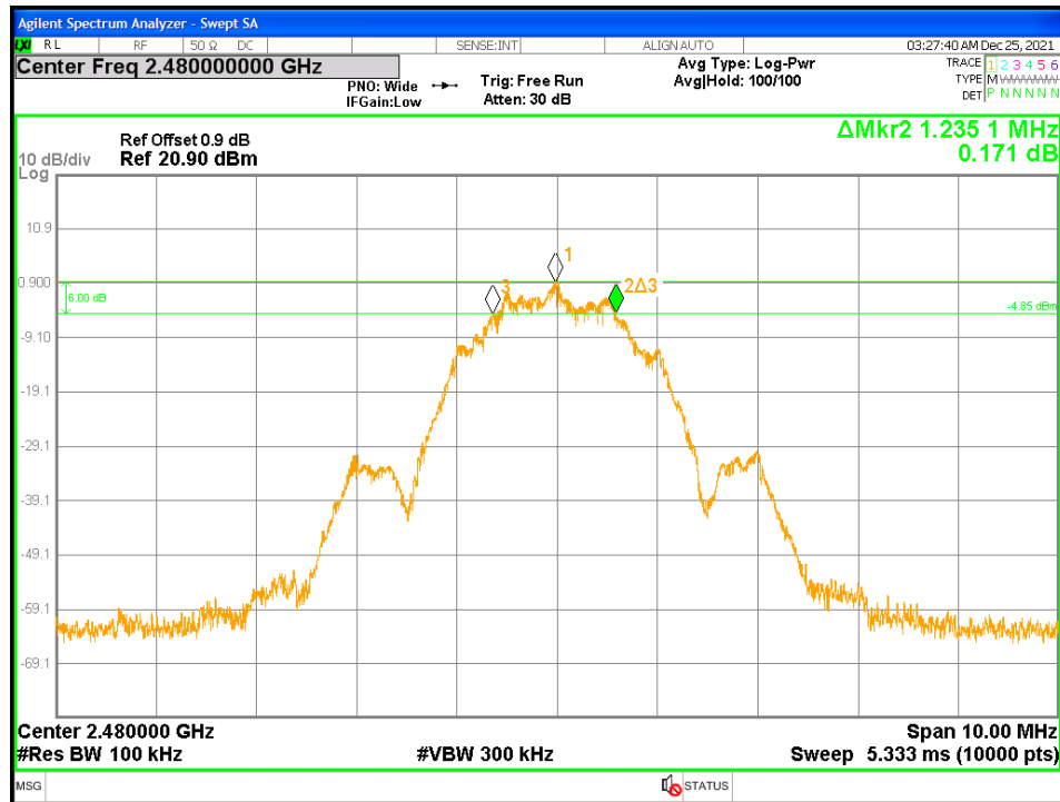
Figure 17: DTS Bandwidth-Headset at 2 Mbps - 2480 MHz
