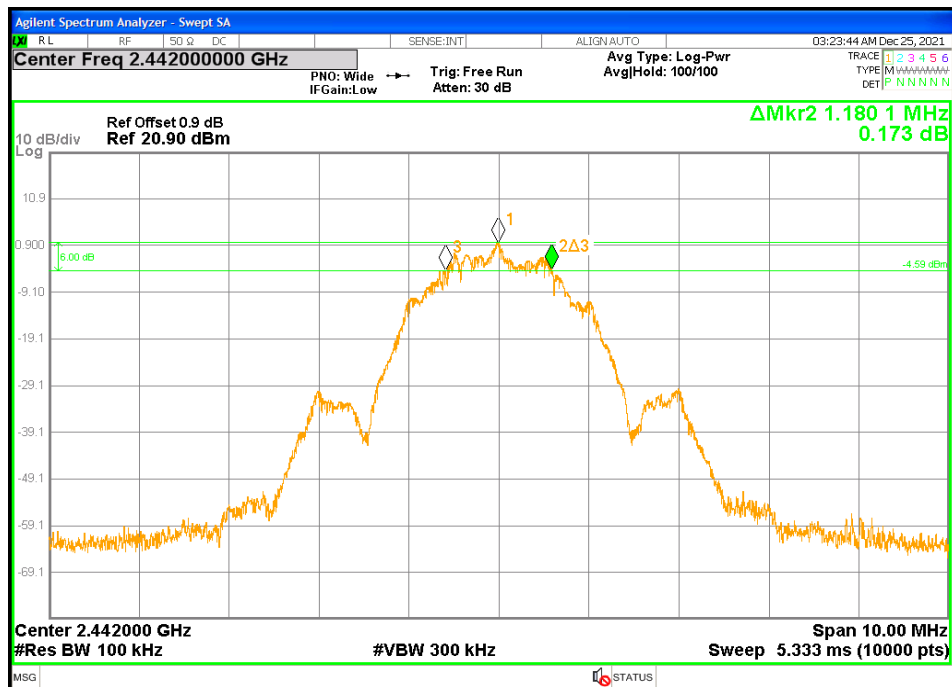
Figure 16: DTS Bandwidth-Headset at 2 Mbps - 2442 MHz
