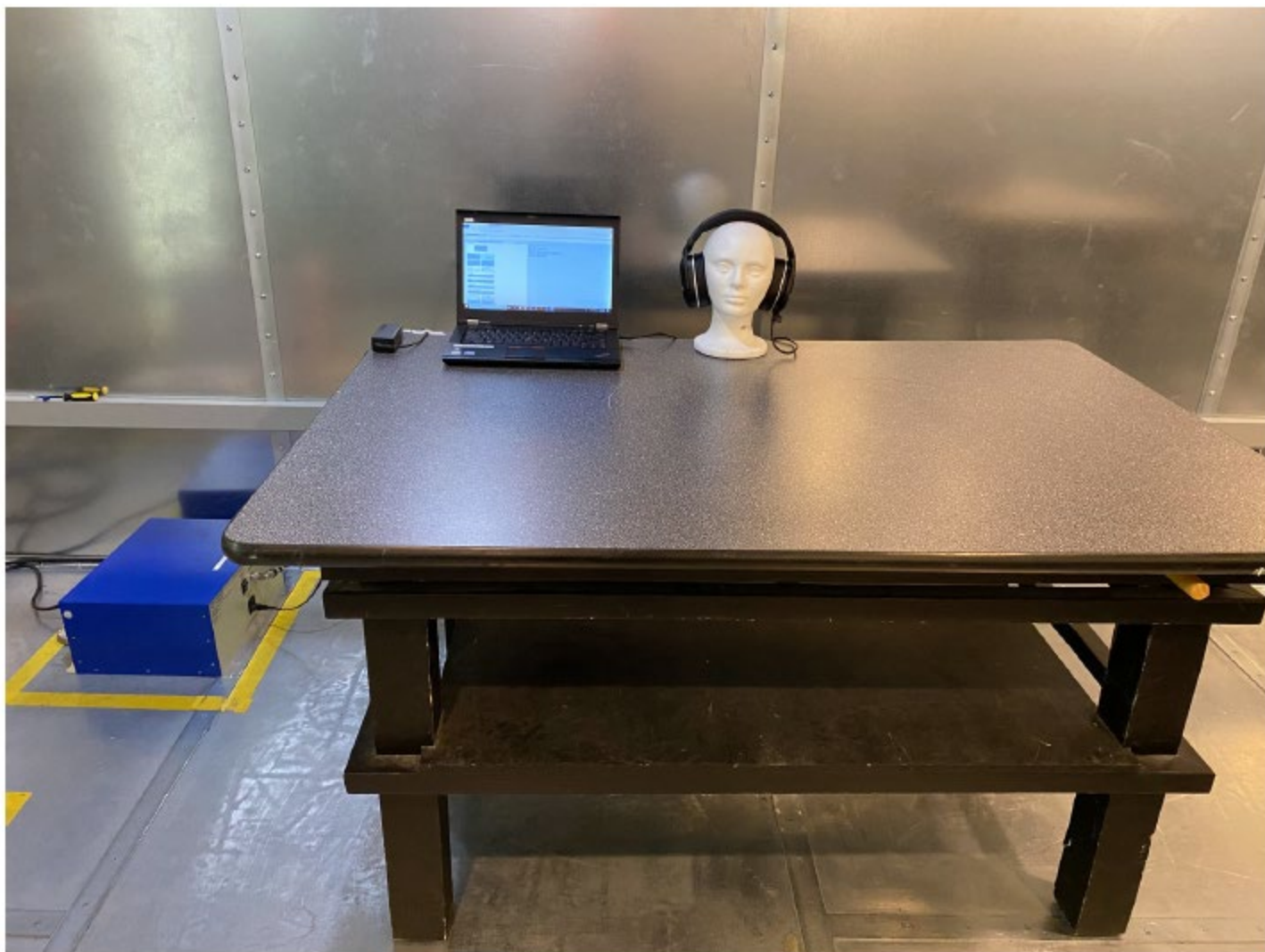
Figure 10: AC Conducted Emission Test Setup (Front View)
