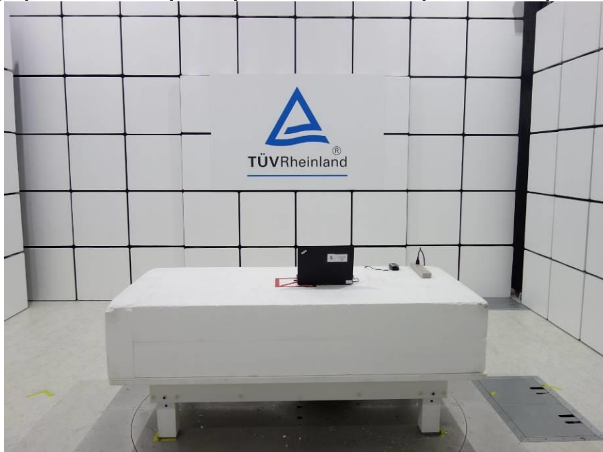
Photograph 1: Test Setup for Spurious Emissions (Front View 1)
