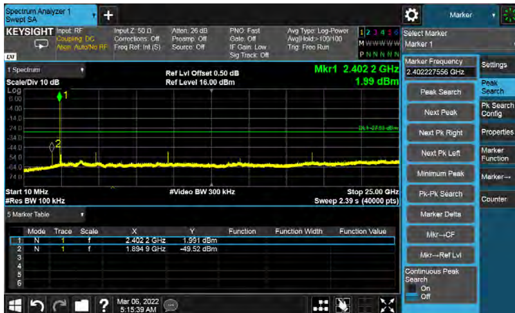
Figure 33: Out of band Emission - 2402 MHz at 2 Mbps
