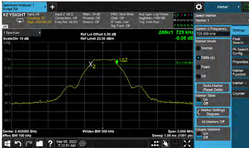
Figure 8: DTS Bandwidth 2402 MHz at 1 Mbps
