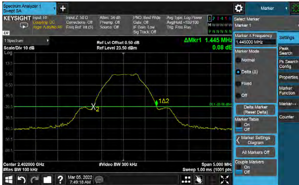
Figure 26: Conducted Band Edge - 2402 MHz at 1 Mbps
