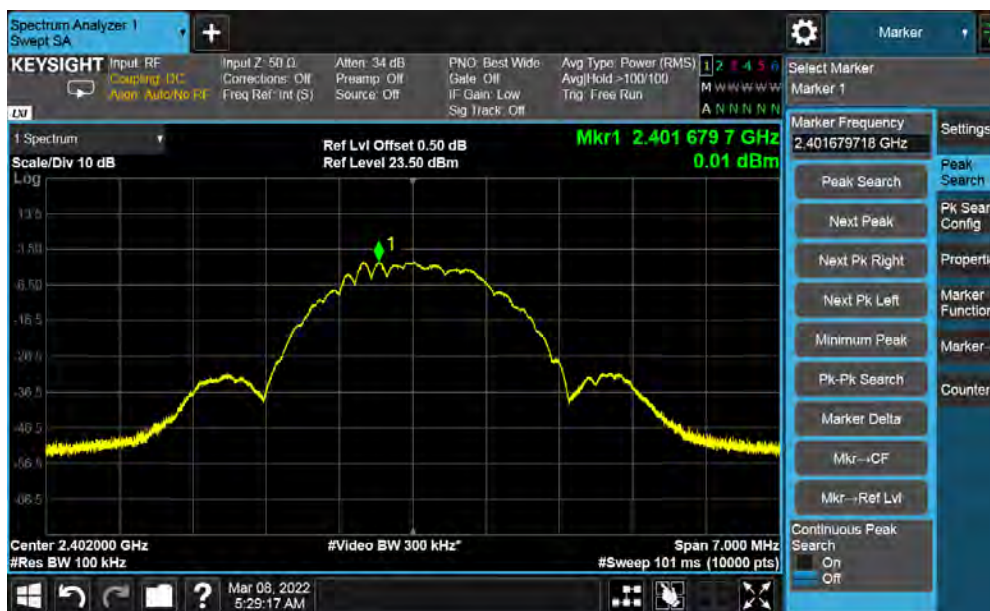
Figure 23: Maximum Power Spectral Density-2402 MHz at 2 Mbps
