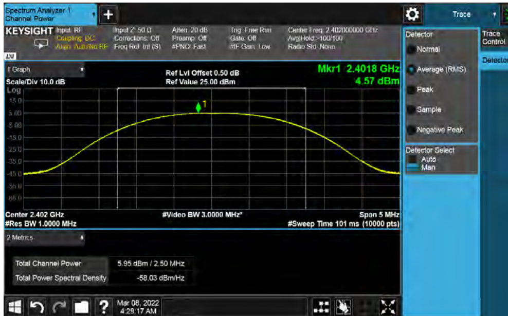
Figure 2: Maximum Transmitted Power, 2402 MHz at 1Mbps
