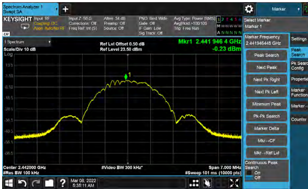
Figure 24: Maximum Power Spectral Density-2442 MHz at 2 Mbps
