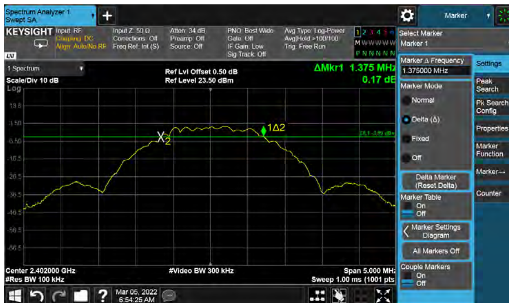
Figure 14: DTS Bandwidth 2402 MHz at 2 Mbps
