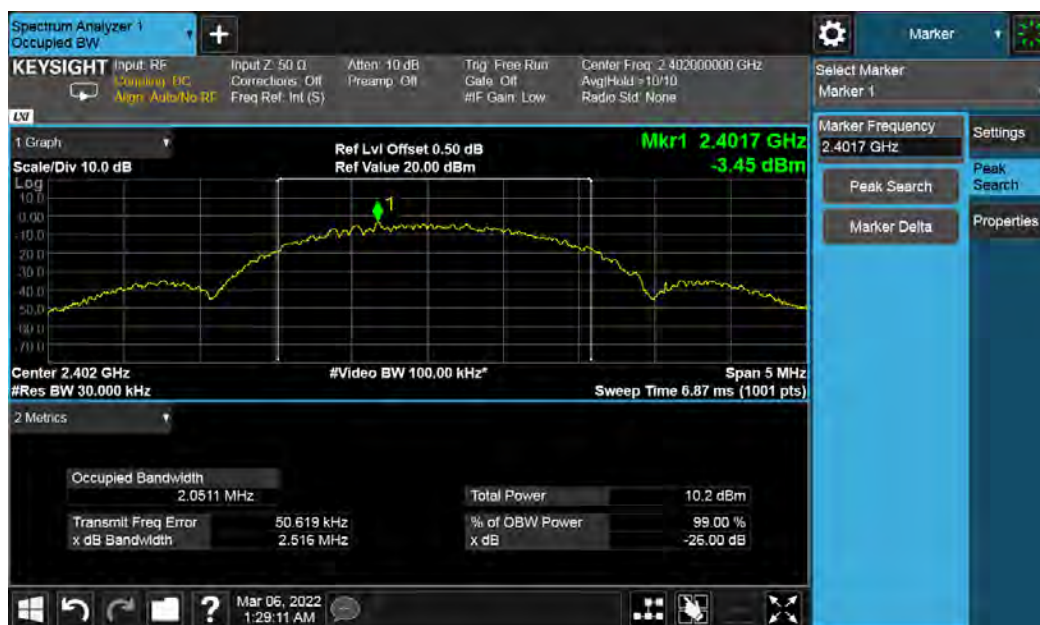
Figure 17: 99% Bandwidth 2402 MHz at 2 Mbps
