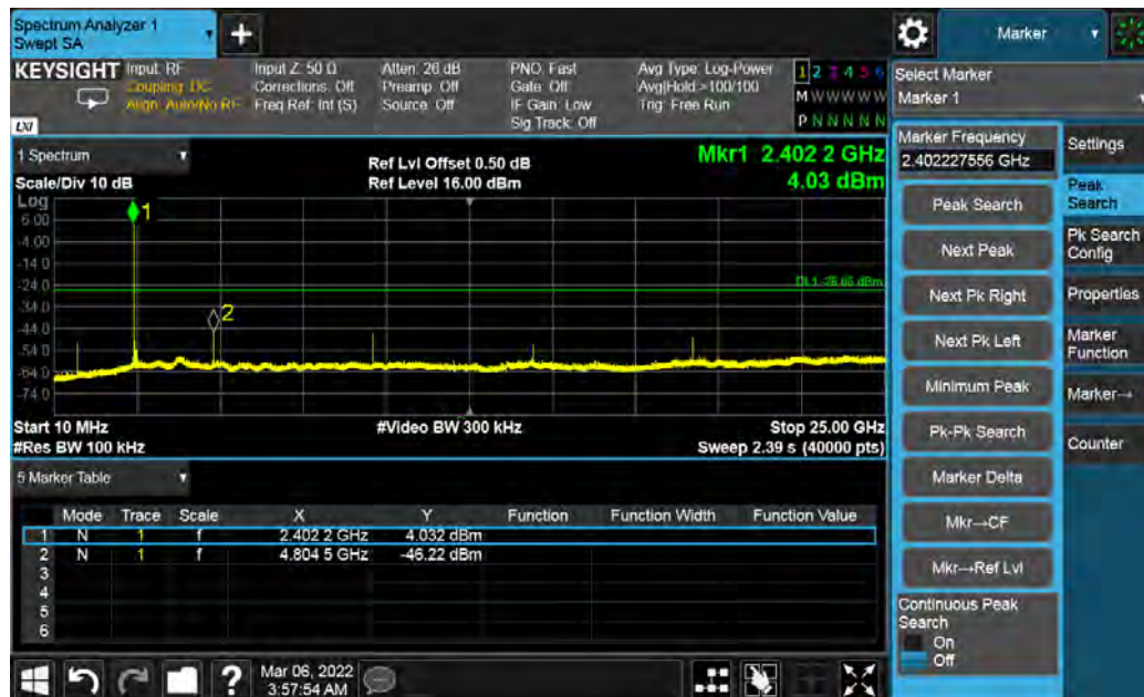
Figure 27: Out of band Emission - 2402 MHz at 1 Mbps
