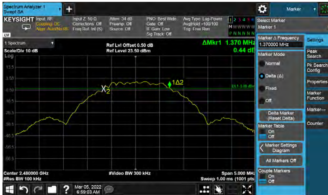
Figure 16: DTS Bandwidth 2480 MHz at 2 Mbps
