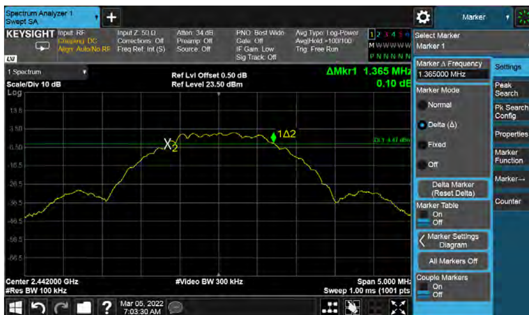
Figure 15: DTS Bandwidth 2442 MHz at 2 Mbps
