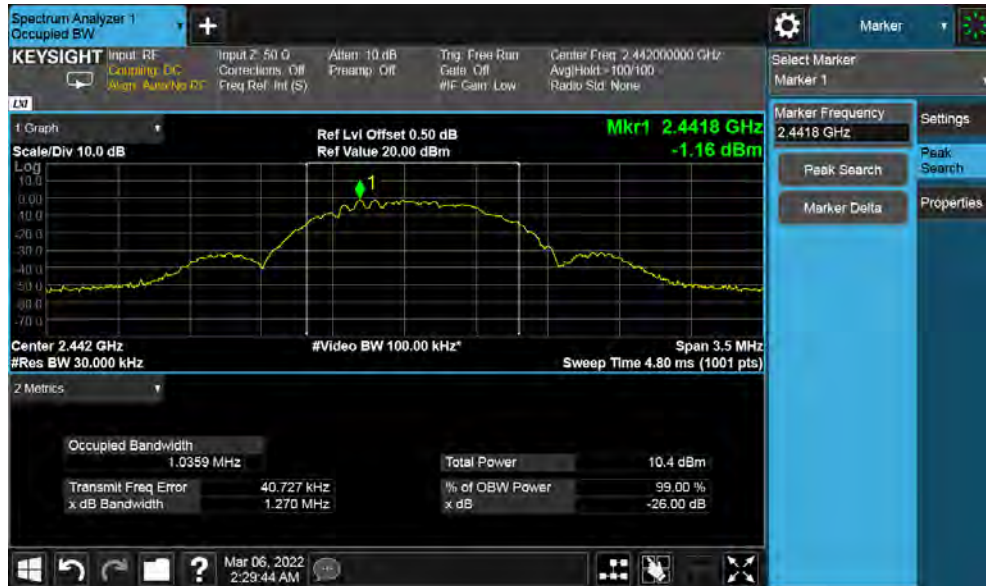
Figure 12: 99% Bandwidth 2442 MHz at 1Mbps
