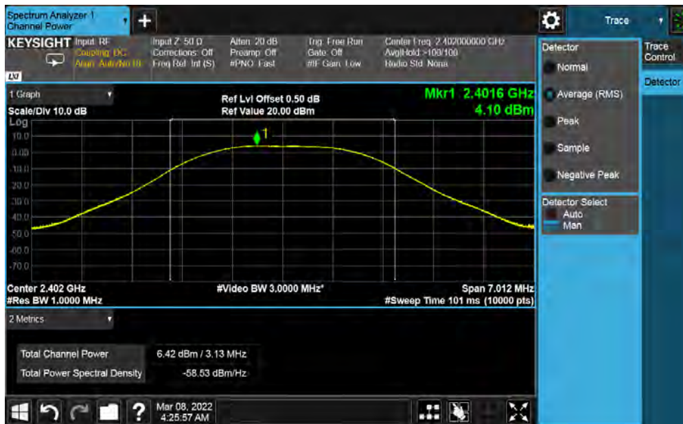
Figure 5: Maximum Conducted Output Power at 2402 MHz at 2Mbps
