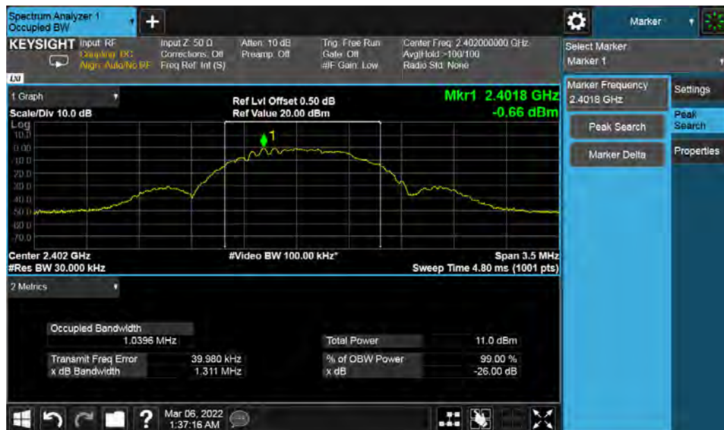
Figure 11: 99% Bandwidth 2402 MHz at 1Mbps
