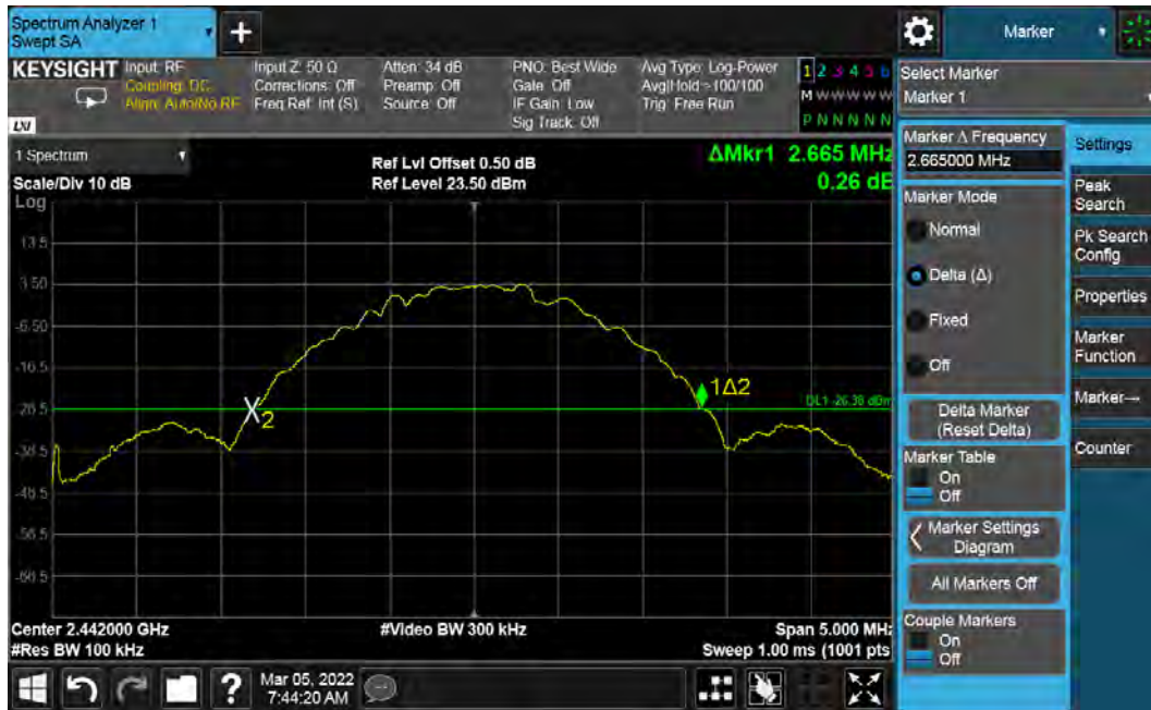
Figure 34: Conducted Band Edge - 2442 MHz at 2 Mbps
