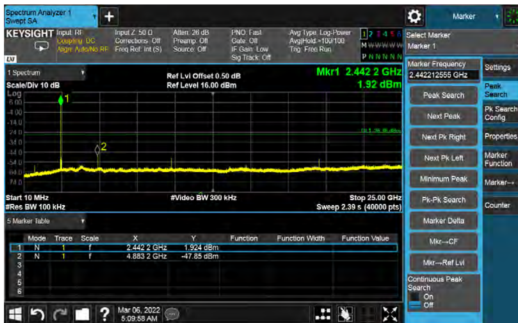
Figure 35: Out of band Emission - 2442 MHz at 2 Mbps
