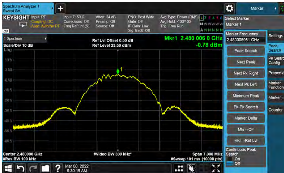
Figure 25: Maximum Power Spectral Density-2480 MHz at 2 Mbps
