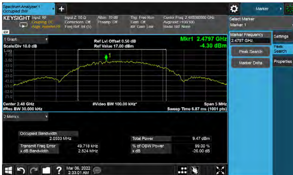
Figure 19: 99% Bandwidth 2480 MHz at 2 Mbps
