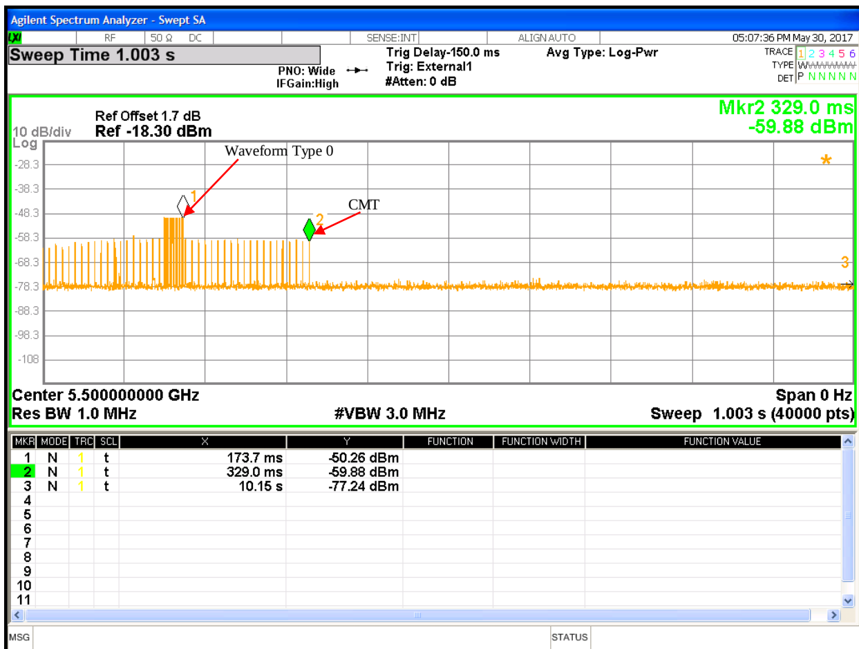
Figure 7: Channel Move Time and Channel Closing Transmission Time using Pulse Radar Waveform 0 at 5500 MHz, 20 MHz Bandwidth (Close-up)
