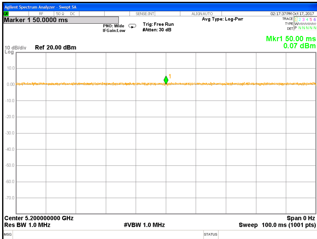
Figure 1: Duty Cycle for 802.11a
