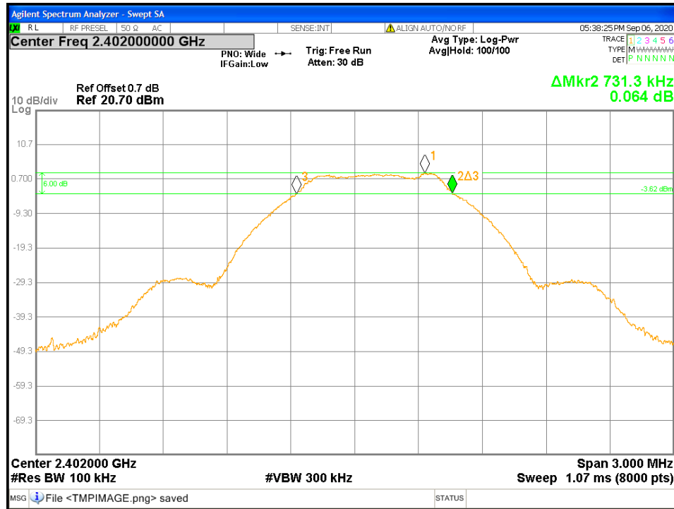
Figure 5: DTS Bandwidth-Headset -2402 MHz
