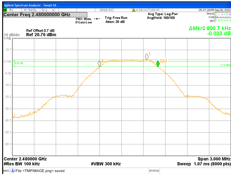
Figure 7: DTS Bandwidth-Headset -2480 MHz
