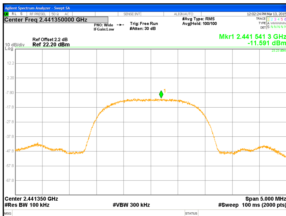
Figure 14: Maximum Power Spectral Density-2441.35MHz- Transmitter
