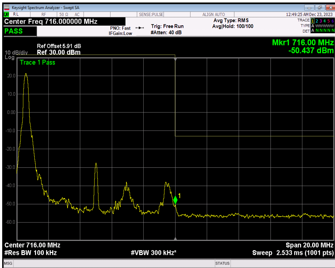
Band17 QPSK BW=10MHz Channel=23800 RB Size=1 Position=#Max
