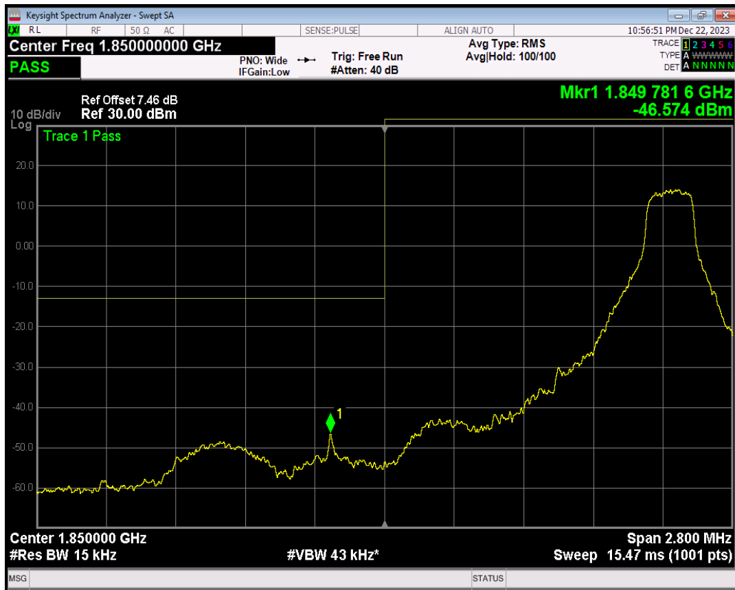
Band2 QPSK BW=1.4MHz Channel=18607 RB Size=6 Position=#0
