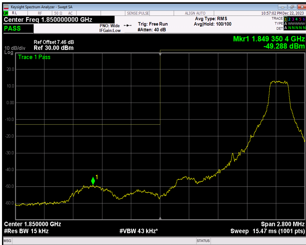
Band2 16QAM BW=1.4MHz Channel=18607 RB Size=6 Position=#0
