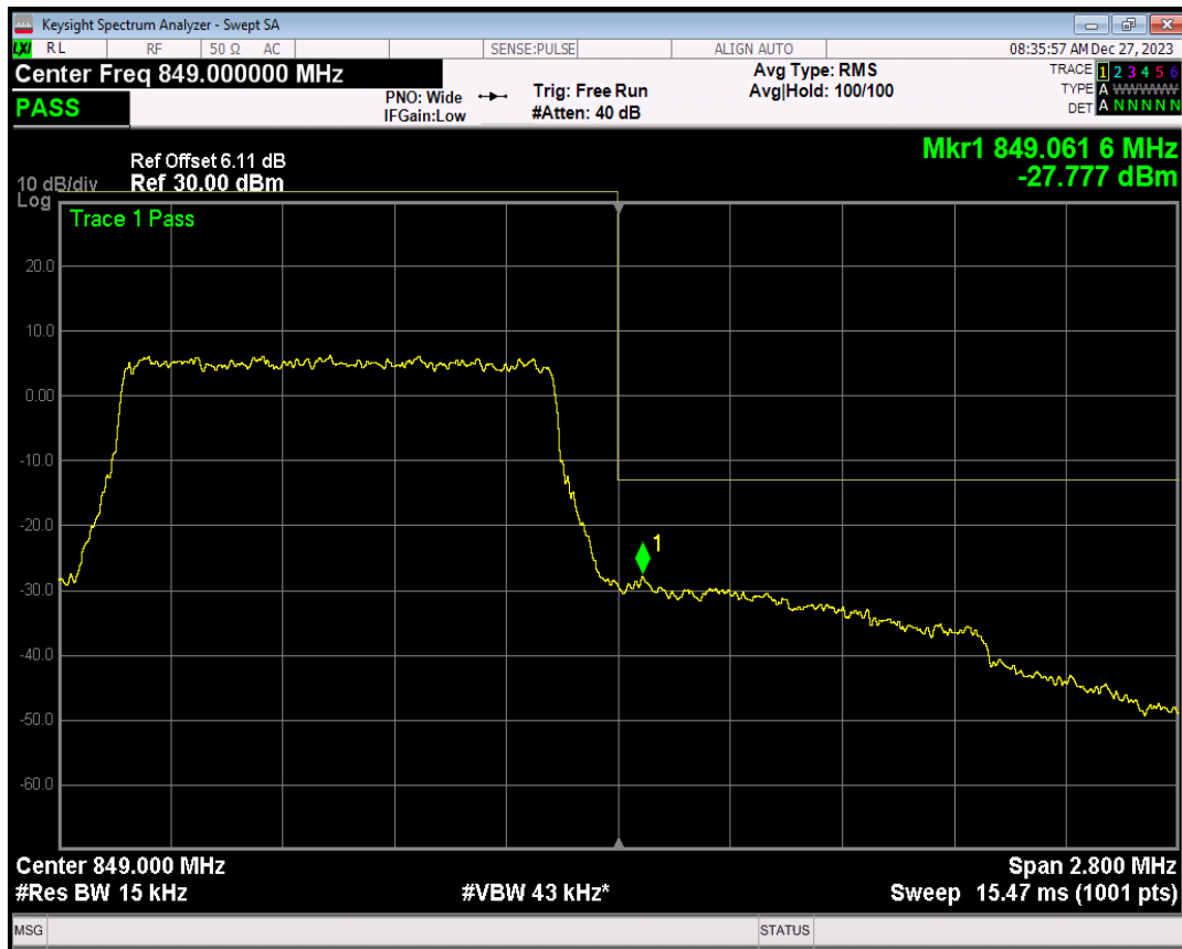
Band26(824-849) 16QAM BW=1.4MHz Channel=27033 RB Size=1 Position=#Max
