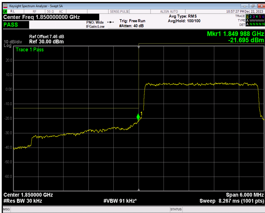
Band2 16QAM BW=3MHz Channel=18615 RB Size=1 Position=#0
