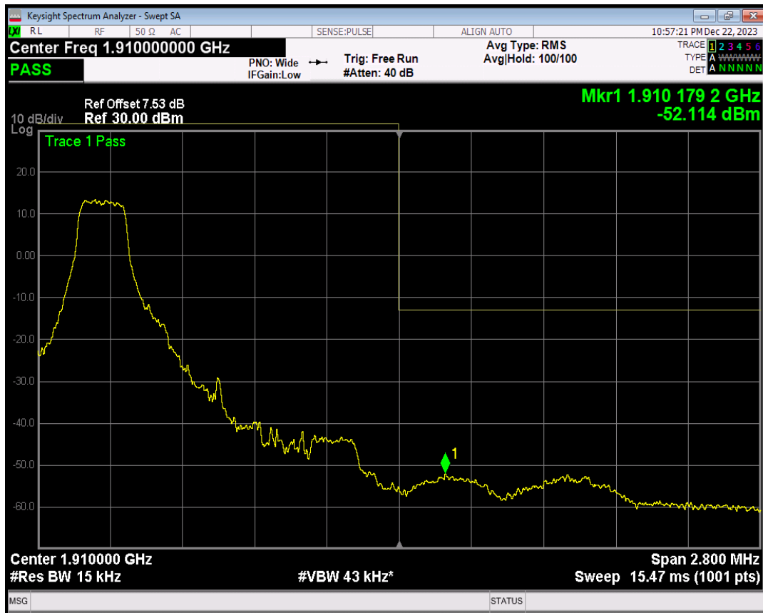
Band2 16QAM BW=1.4MHz Channel=19193 RB Size=1 Position=#Max
