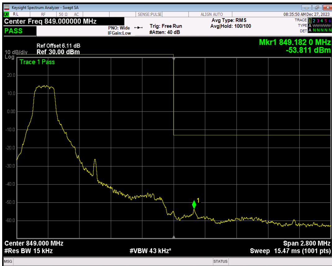
Band26(824-849) QPSK BW=1.4MHz Channel=27033 RB Size=1 Position=#Max
