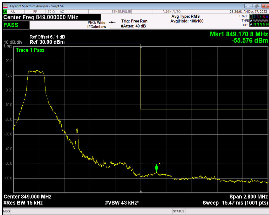
Band26(824-849) QPSK BW=1.4MHz Channel=27033 RB Size=6 Position=#0
