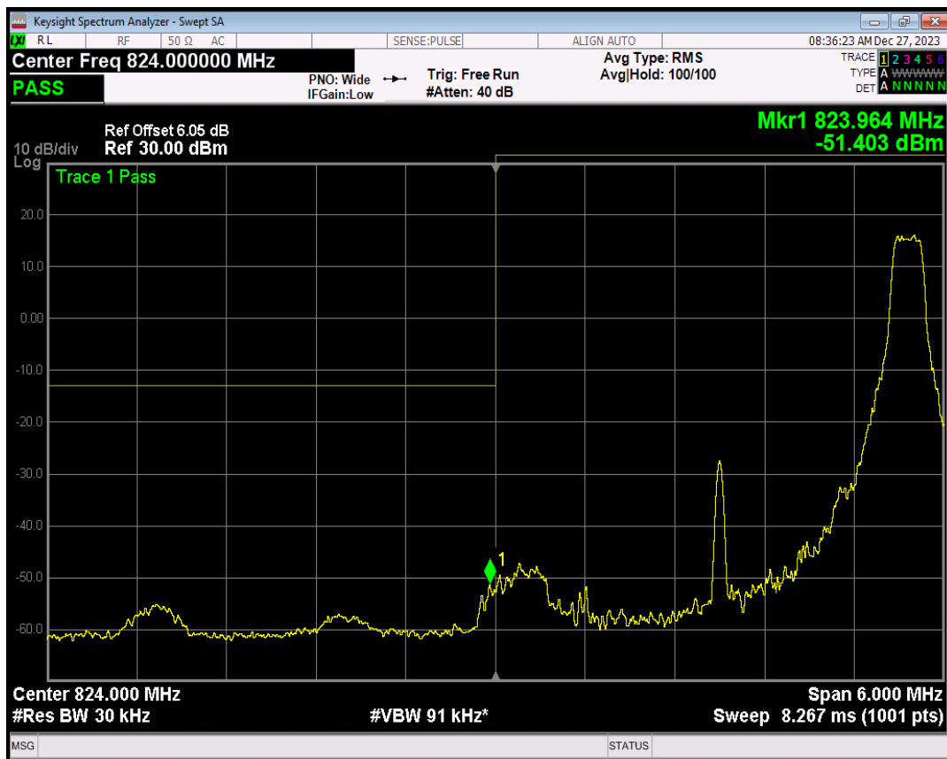
Band26(824-849) 16QAM BW=3MHz Channel=26805 RB Size=15 Position=#0
