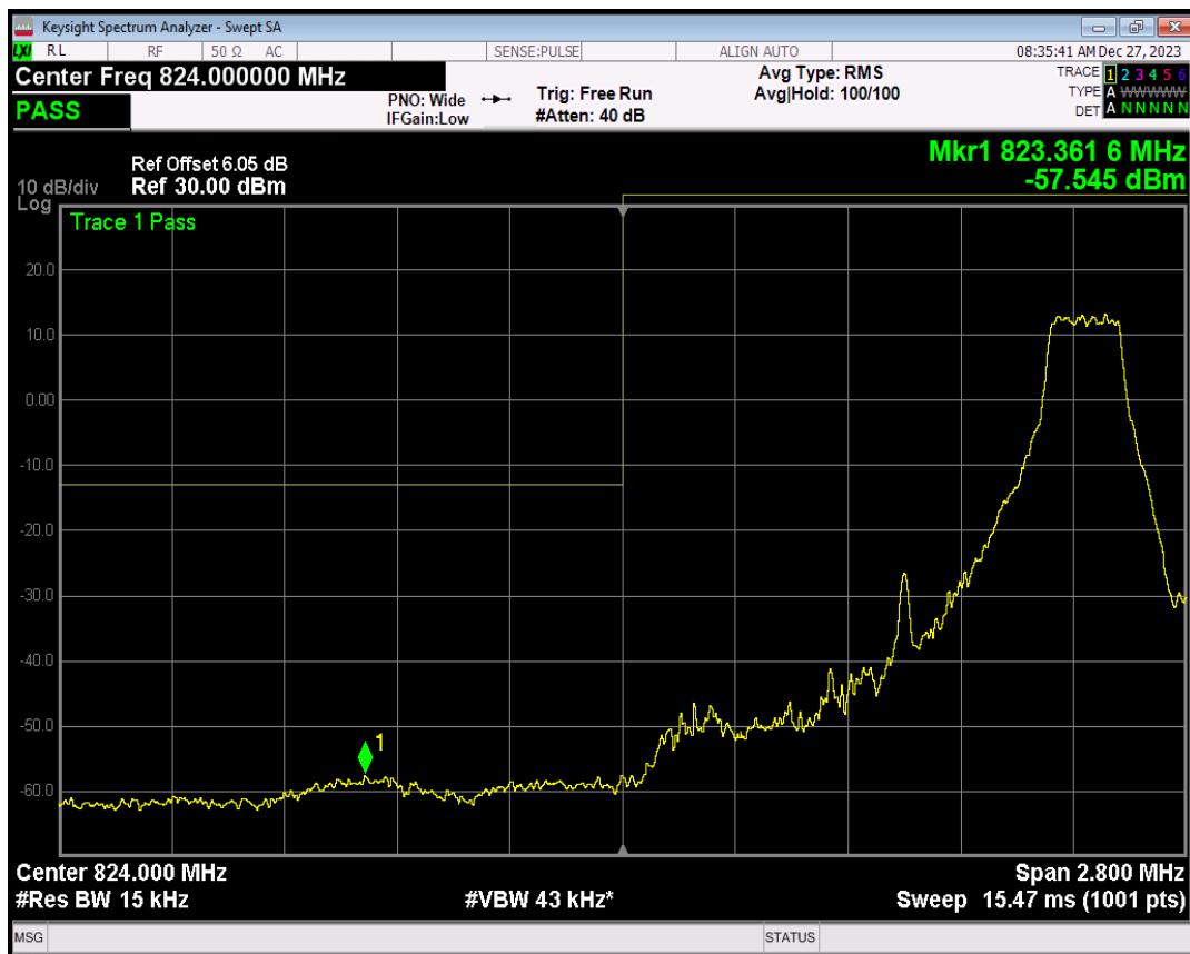
Band26(824-849) 16QAM BW=1.4MHz Channel=26797 RB Size=6 Position=#0
