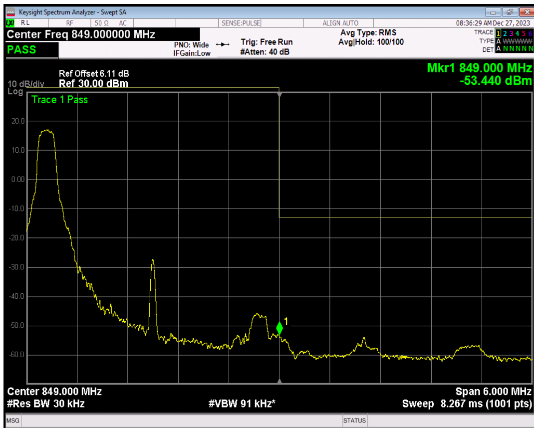
Band26(824-849) QPSK BW=3MHz Channel=27025 RB Size=1 Position=#Max
