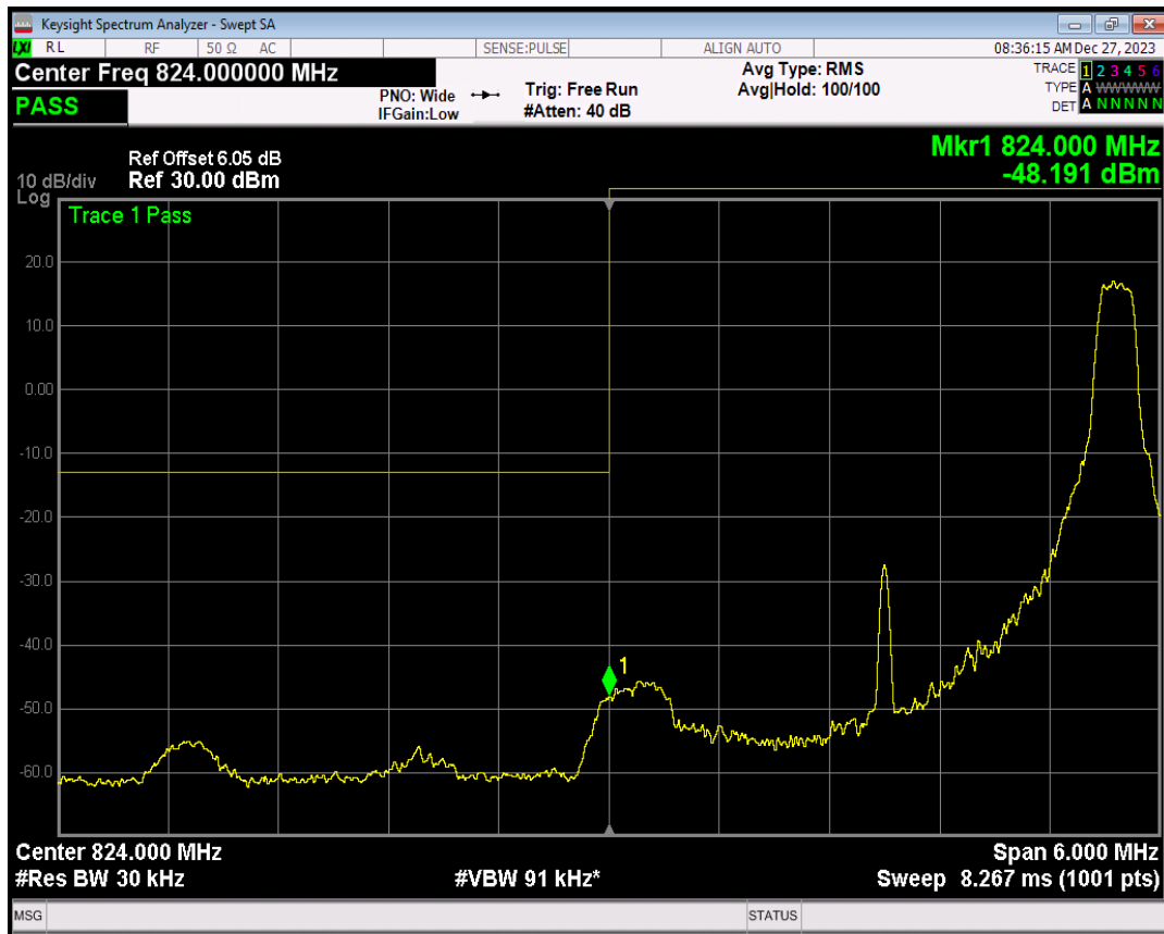
Band26(824-849) QPSK BW=3MHz Channel=26805 RB Size=15 Position=#0
