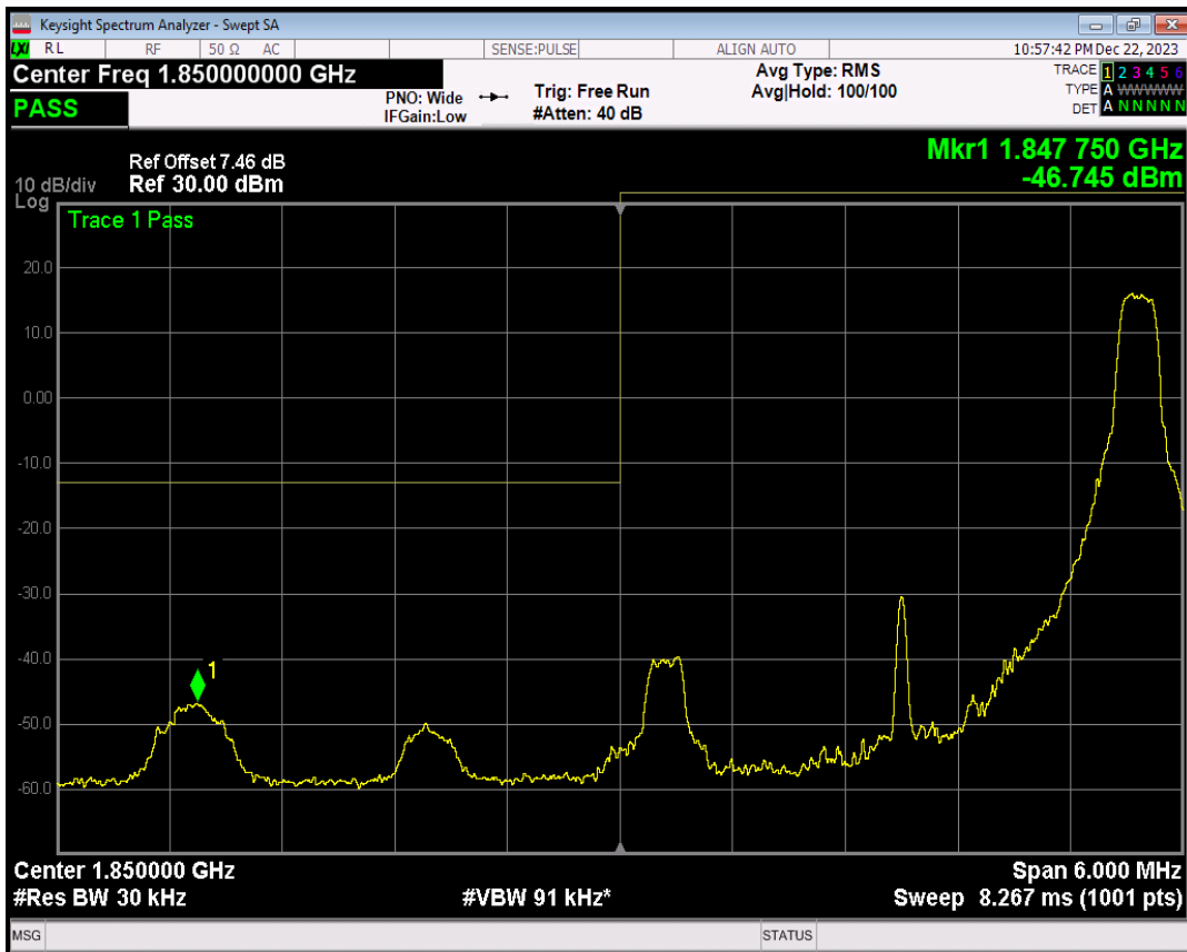
Band2 16QAM BW=3MHz Channel=18615 RB Size=15 Position=#0
