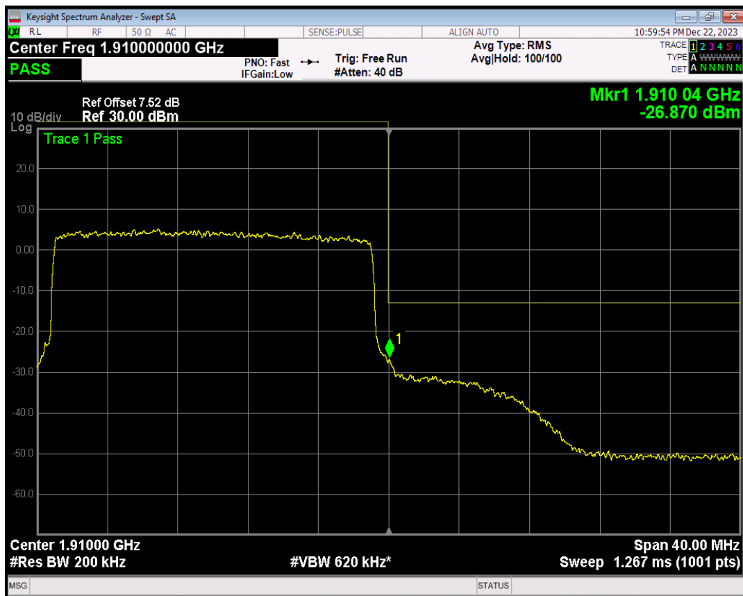
Band2 16QAM BW=20MHz Channel=19100 RB Size=1 Position=#0
