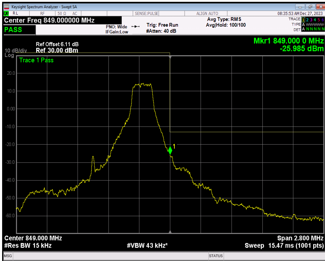
Band26(824-849) 16QAM BW=1.4MHz Channel=27033 RB Size=1 Position=#0
