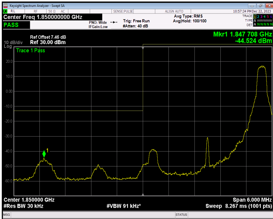
Band2 QPSK BW=3MHz Channel=18615 RB Size=15 Position=#0
