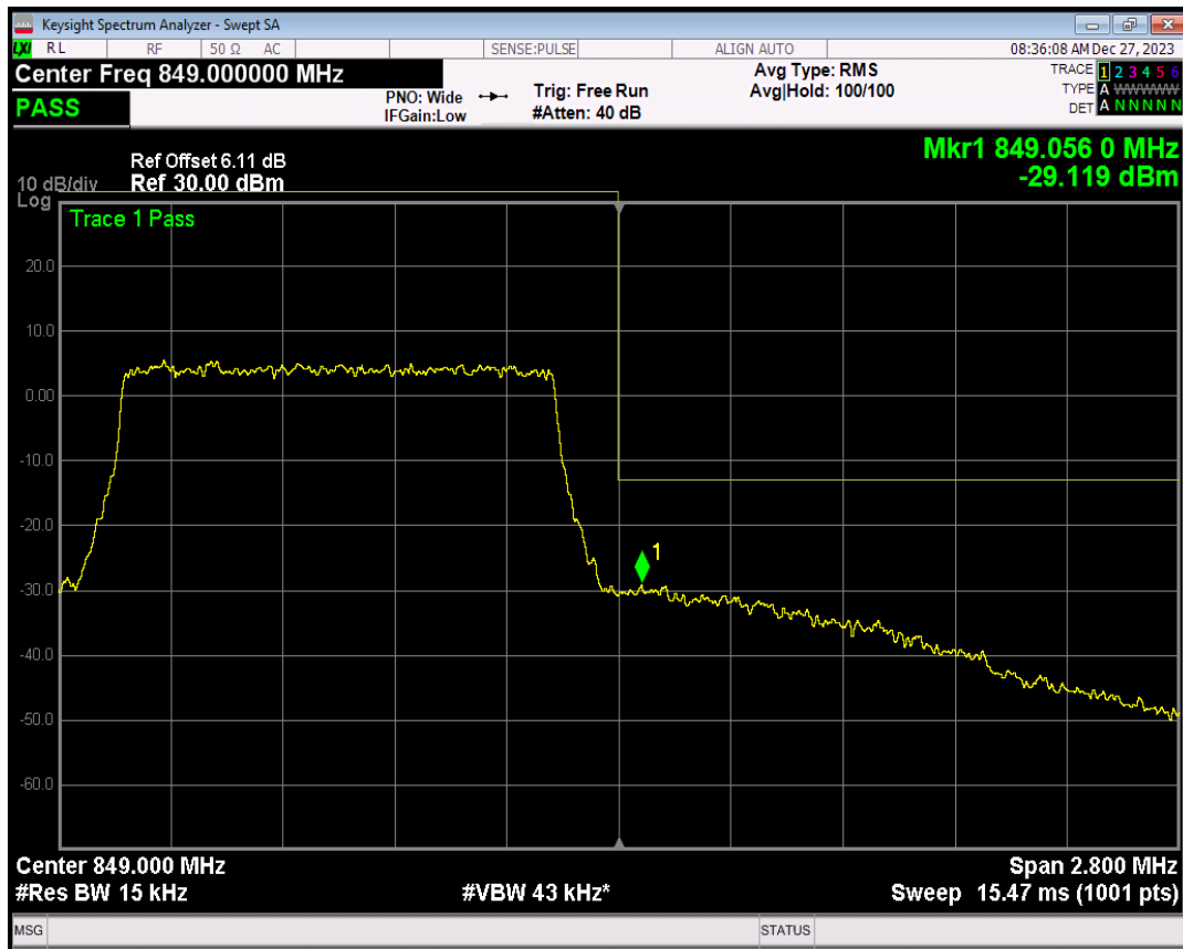
Band26(824-849) QPSK BW=3MHz Channel=26805 RB Size=1 Position=#0
