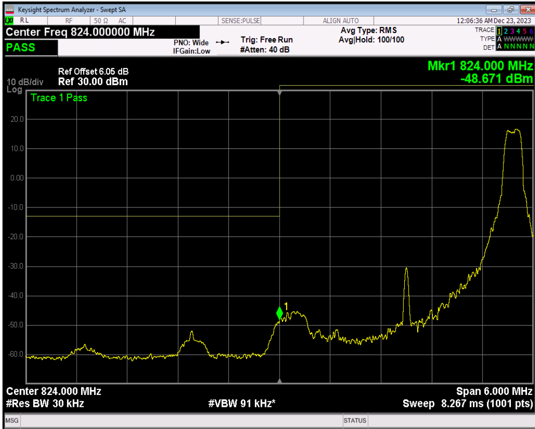
Band5 QPSK BW=3MHz Channel=20415 RB Size=15 Position=#0
