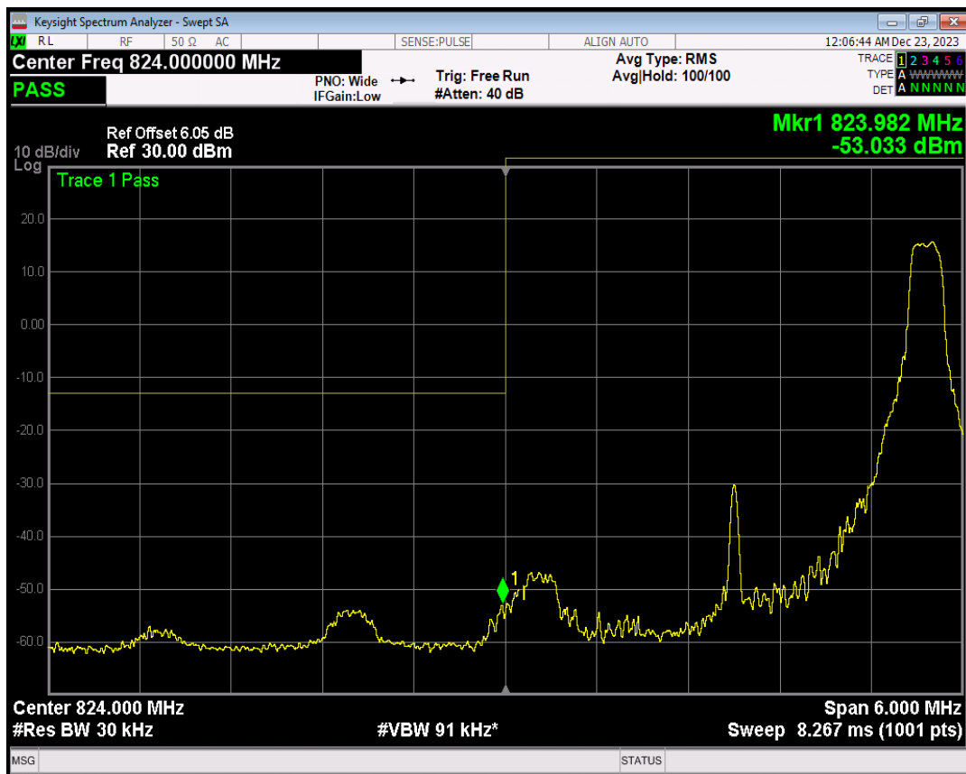
Band5 16QAM BW=3MHz Channel=20415 RB Size=15 Position=#0
