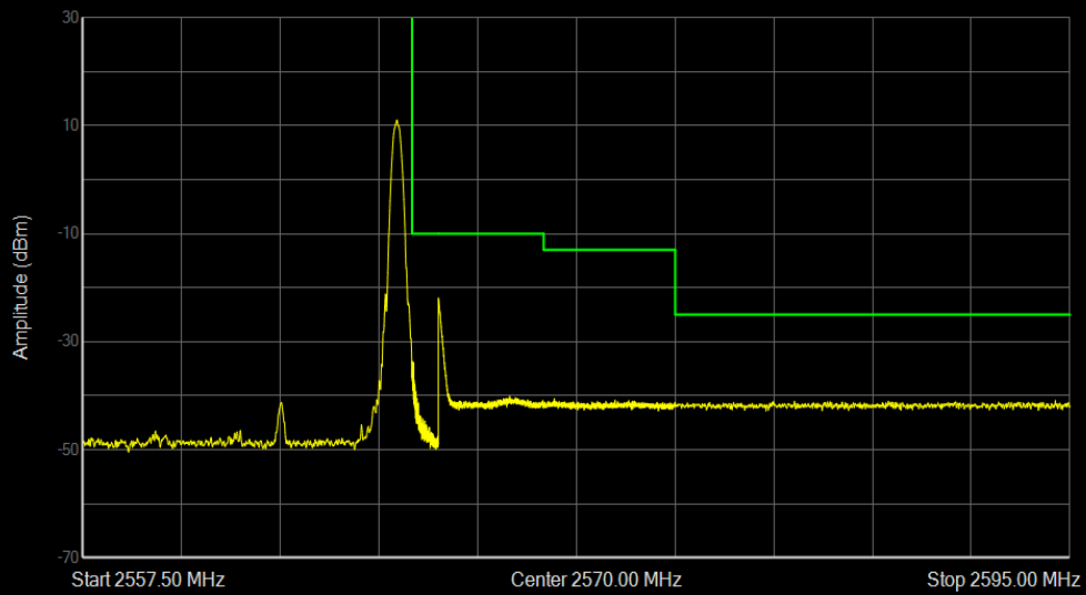
Band7 QPSK BW=10MHz Channel=21400 RB Size=1 Position=#Max
