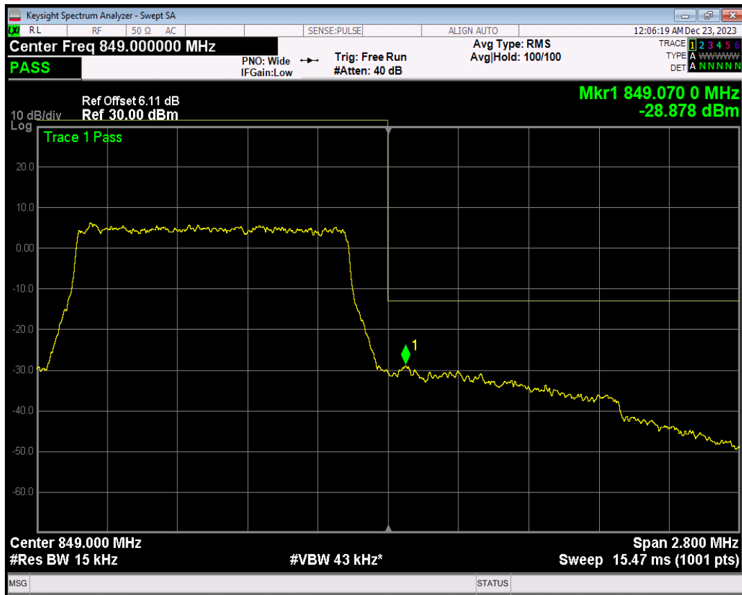
Band5 16QAM BW=1.4MHz Channel=20643 RB Size=1 Position=#Max
