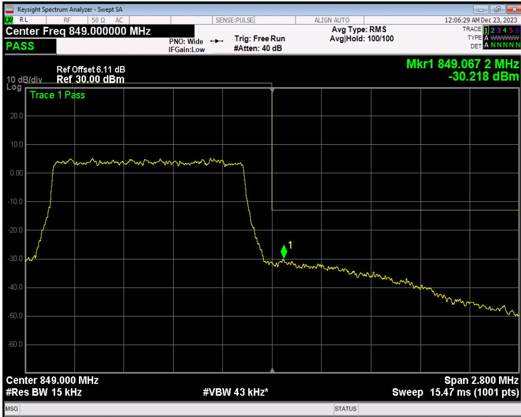
Band5 QPSK BW=3MHz Channel=20415 RB Size=1 Position=#0
