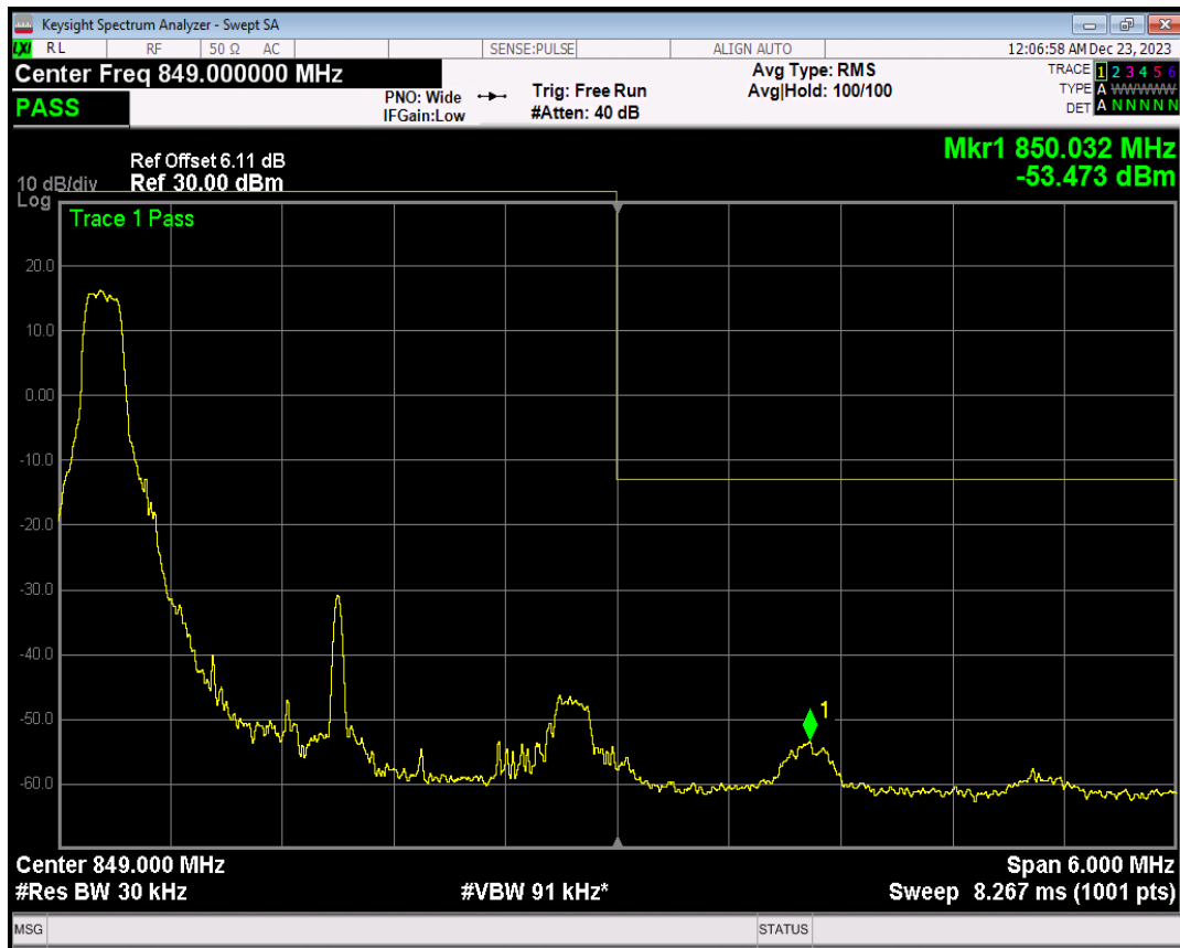
Band5 16QAM BW=3MHz Channel=20635 RB Size=1 Position=#Max
