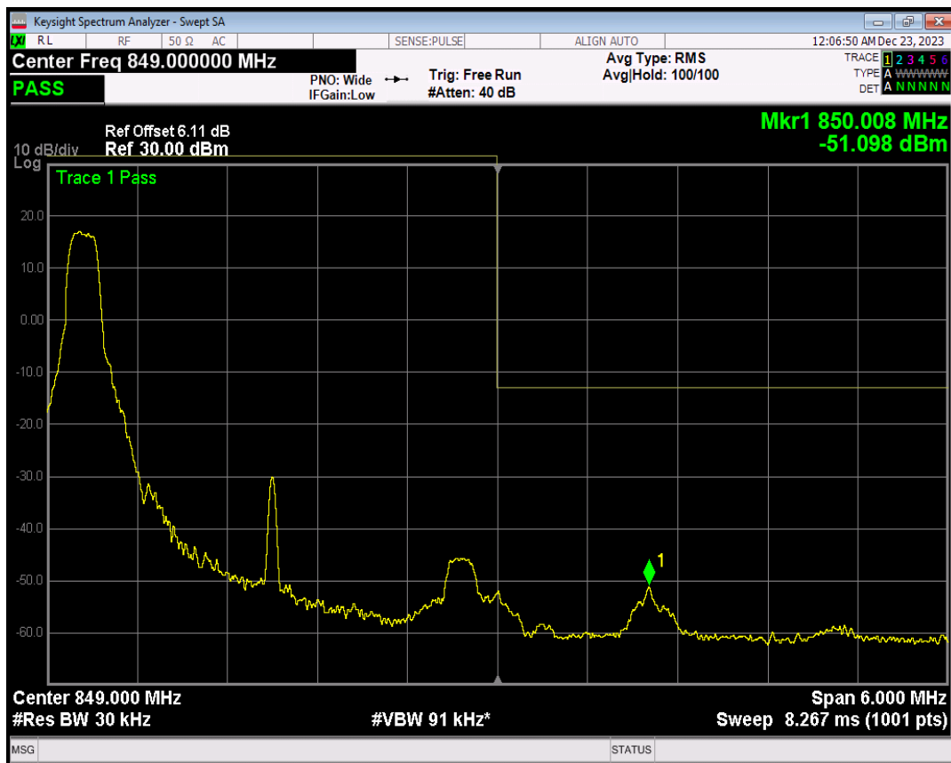
Band5 QPSK BW=3MHz Channel=20635 RB Size=1 Position=#Max
