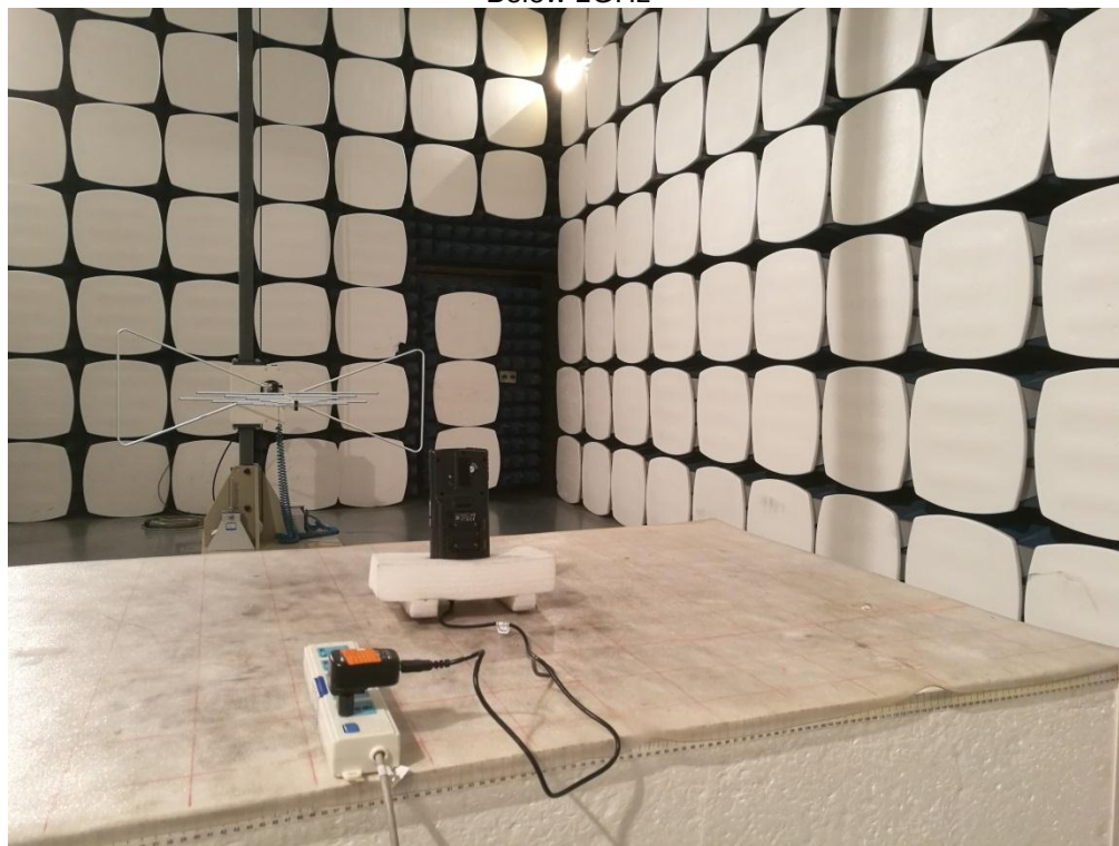
Radiated Spurious Emission Below 1GHz
