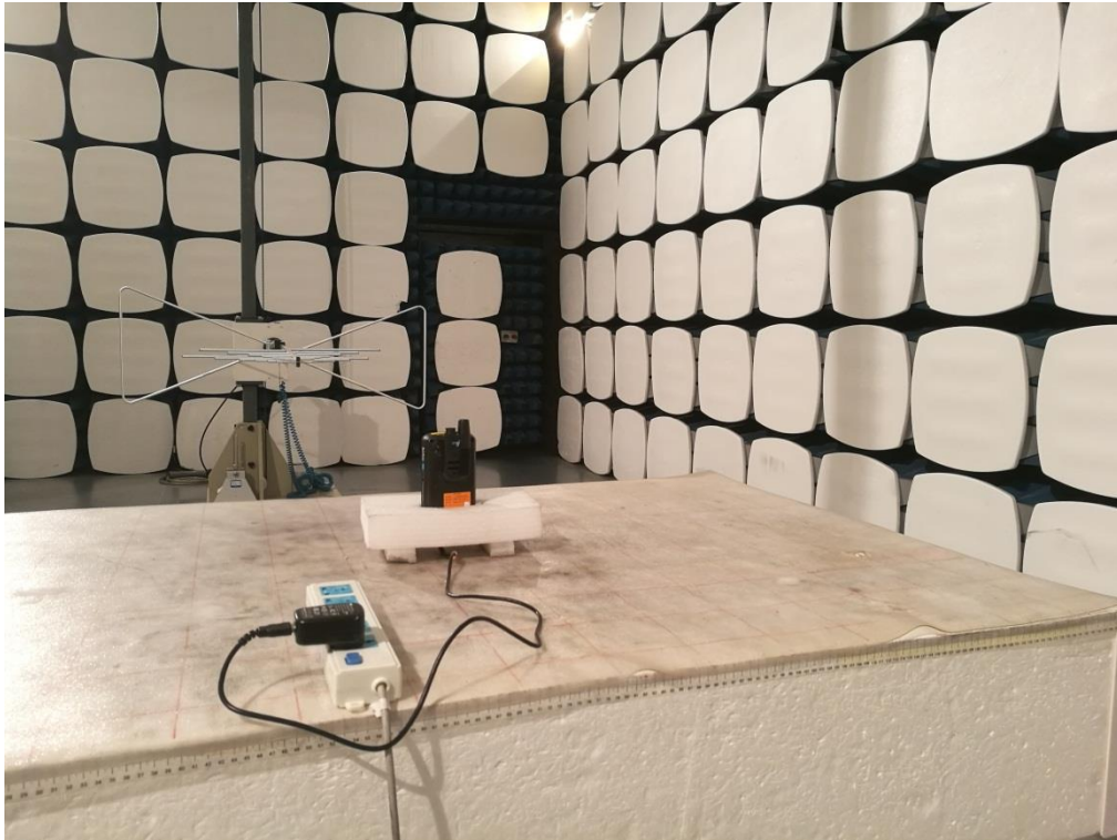
Radiated Spurious Emission Below 1GHz
